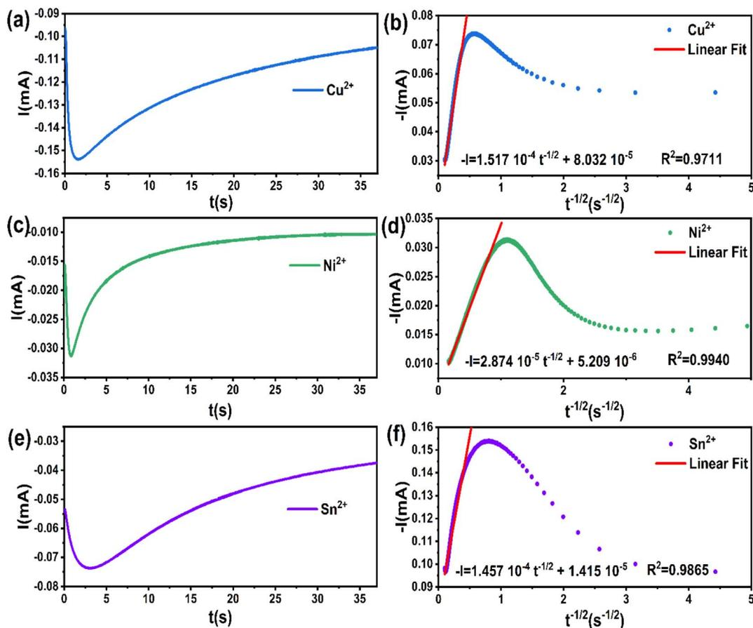
Fig. 5 Transients current and their plots according to the Cottrell equation for: (a and b)  $\text{Cu}^{2+}$ , (c and d)  $\text{Ni}^{2+}$  and (e and f)  $\text{Sn}^{2+}$ . The potentials applied are  $-0.62$  V,  $-1.10$  V and  $-1.05$  V for  $\text{Cu}^{2+}$ ,  $\text{Ni}^{2+}$  and  $\text{Sn}^{2+}$  respectively.
