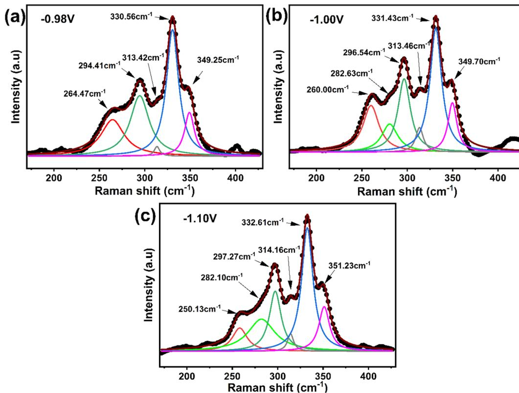
Fig. 13 Raman spectra analysis of sulfurized CNTS thin films electrodeposited at different potentials: (a)  $-0.98\text{ V}$ , (b)  $-1.00\text{ V}$  and (c)  $-1.10\text{ V}$ .
