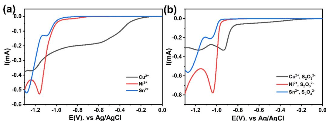
Fig. 3 Cathodic polarization curves of CNT precursor on FTO electrode in the electrolytic bath containing  $\text{Na}_3\text{C}_6\text{H}_5\text{O}_7$  under the following conditions: (a) without  $\text{S}_2\text{O}_3^{2-}$ , (b) with  $\text{S}_2\text{O}_3^{2-}$ , rate scan ( $25 \text{ mV s}^{-1}$ ), potential range (0 V to  $-1.3 \text{ V}$ . vs. Ag/AgCl), pH = 5.5.
