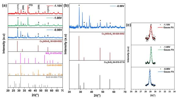
Fig. 12 (a) XRD patterns of CNTS sulfurized films at different applied potentials, (b) XRD patterns of CNTS film obtained at -0.98 V and (c) the mean peak intensity of 112 reflections.
