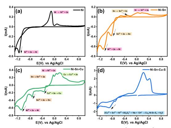
Fig. 2 Cyclic voltammograms of CNTS precursor in bath electrolytic containing  $Na_3C_6H_5O_7$ : (a)  $Ni^{2+}$  (0.035 M), (b)  $Ni^{2+}$  (0.035 M) +  $Sn^{2+}$  (0.015 M), (c)  $Ni^{2+}$  (0.035 M) +  $Sn^{2+}$  (0.015 M). Scan rate (25 mV s<sup>-1</sup>), potential range (1 to -1.3 V. vs. Ag/AgCl), pH = 5.5.
