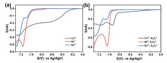
Fig. 3 Cathodic polarization curves of CNT precursor on FTO electrode in the electrolytic bath containing  $Na_3C_6H_5O_7$  under the following conditions: (a) without  $S_2O_3^{2-}$ , (b) with  $S_2O_3^{2-}$ , rate scan (25 mV s<sup>-1</sup>), potential range (0 V to -1.3 V. vs. Ag/AgCl), pH = 5.5.
