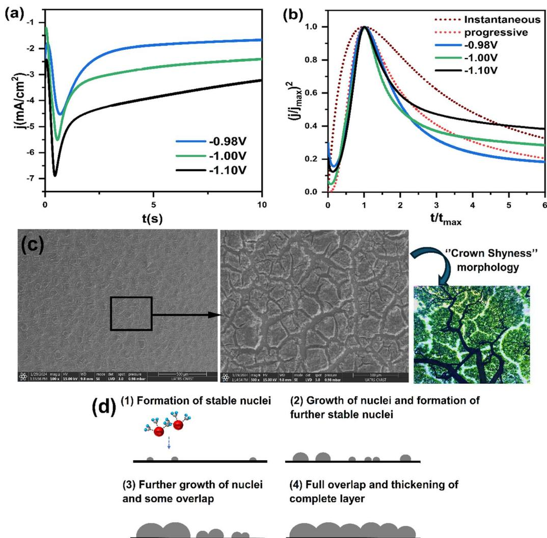
Fig. 8 (a) Transients current of CNTS precursor at different applied potentials, (b) the corresponding Scharifker–Hills' models, (c) SEM images of as deposited CNTS film deposited at  $-0.98$  V, and (d) mechanism involving progressive nucleation and growth as hemispherical centers.
