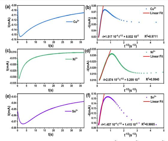
Fig. 5 Transients current and their plots according to the Cottrell equation for: (a and b)  $Cu^{2+}$ , (c and d)  $Ni^{2+}$  and (e and f)  $Sn^{2+}$ . The potentials applied are -0.62 V, -1.10 V and -1.05 V for  $\text{Cu}^{2+}$ ,  $\text{Ni}^{2+}$  and  $\text{Sn}^{2+}$  respectively.
