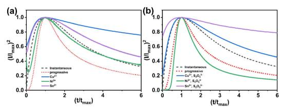
Fig. 7 Theoretical plots of instantaneous and progressive nucleation processes and experimental plots of: (a) CNT precursor, (b) CNT precursor in presence of  $S_2O_3^{2-}$ .
