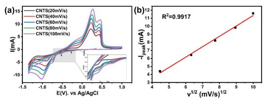
Fig. 4 (a) Cyclic voltammograms of CNTS precursor on FTO electrode at different scan rate, (b) linear plots of cathodic peak (Ipeak) current as a function of the square root of scan rate  $(v^{1/2})$ .
