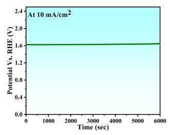
Fig. 10 Chronopotentiometry curve for NCHNF at 10 mA cm<sup>-2</sup>.
