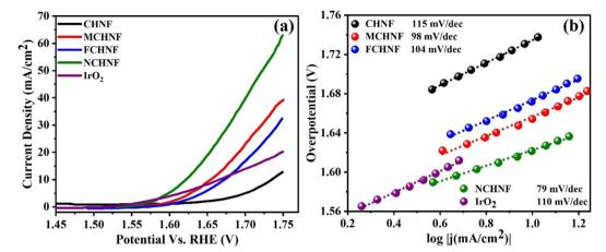
Fig. 7 (a) LSV polarization curves using OHNF, MCHNF, FCHNF and NCHNF electrocatalysts and their corresponding (b) Tafel slopes.
