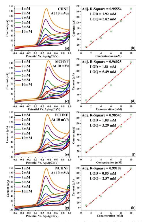
Fig. 11 Cyclic voltammograms at different molar concentrations of ascorbic acid ranging from 1 to 10 mM using (a). CHNF, (c). MCHNF, (e). FCHNF and (g). NCHNF with their corresponding *R*-square, LOD and LOQ values (b, d, f, and h).
