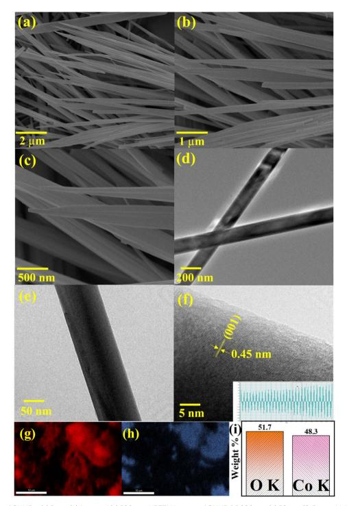
Fig. 4 SEM images of CHNF at (a)  $2 \mu m$ , (b)  $1 \mu m$  and (c) 500 nm, HRTEM images of CHNF, (d) 200 nm, (e) 50 nm, (f), 5 nm with inverse FFT pattern in the inset, (g and h) elemental mapping for  $Co(OH)_2$  with O K and Co K and (i) weight percentage as per EDX analysis.
