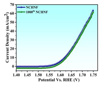
Fig. 9 Stability of NCHNF after 1000 cycles.
