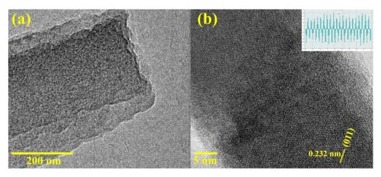
Fig. 6 HRTEM images of NCHNF at (a) 200 nm and (b) 5 nm.
