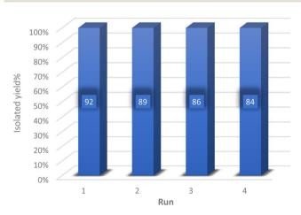
Fig. 8 Ability to recycle and reuse Zn/Cr-LDH@PTRMS@NDBD@Cul catalyst.
