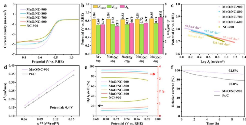
Fig. 5 ORR performance of MnO/NC nanohybrids and NC-900: (a) LSV curves in O $_2$ -saturated 0.1 M KOH at 5 mV s $^{-1}$ ; (b)  $E_{\text{onset}}$ ,  $E_{1/2}$  and  $J_L$  values; (c) Tafel plots derived from the corresponding LSVs. (d) K–L plots of MnO/NC-900 and Pt/C at 0.4 V. (e) H $_2$ O $_2$  yield and  $n$  of MnO/NC nanohybrids and NC-900. (f) Chronoamperometric tests of MnO/NC-900 and Pt/C in O $_2$ -saturated KOH (0.1 M).
