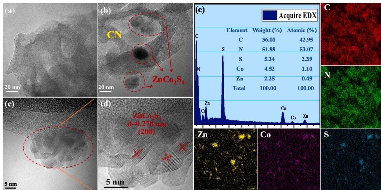
Fig. 4 TEM images of (a) CN and (b)  $\text{ZnCo}_2\text{S}_4/\text{CN}$ , HRTEM images of (c–d)  $\text{ZnCo}_2\text{S}_4/\text{CN}$ , and (e) EDS spectrum of  $\text{ZnCo}_2\text{S}_4/\text{CN}$  and elemental mapping analysis, reprinted with the permission of ref. 132, copyright 2024, Elsevier.
