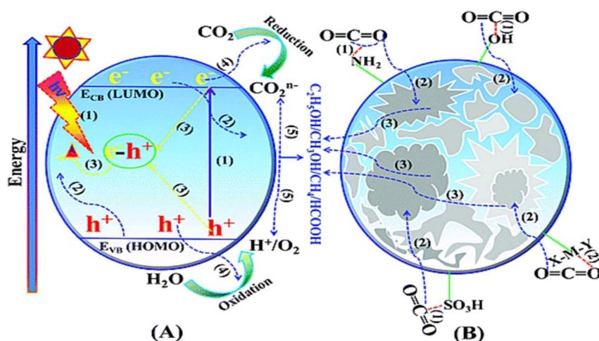
Fig. 12 General steps involved in CO<sub>2</sub> photoreduction coupled with water oxidation: (A) optoelectronic: (1) e<sup>-</sup>-h<sup>+</sup> generation, (2) charge migration to the surface, (3) e<sup>-</sup>-h<sup>+</sup> recombination, (4) CO<sub>2</sub> photoreduction, (B) physicochemical: (1) CO<sub>2</sub> adsorption, (2) CO<sub>2</sub> activation, and (3) product desorption.<sup>257</sup>
