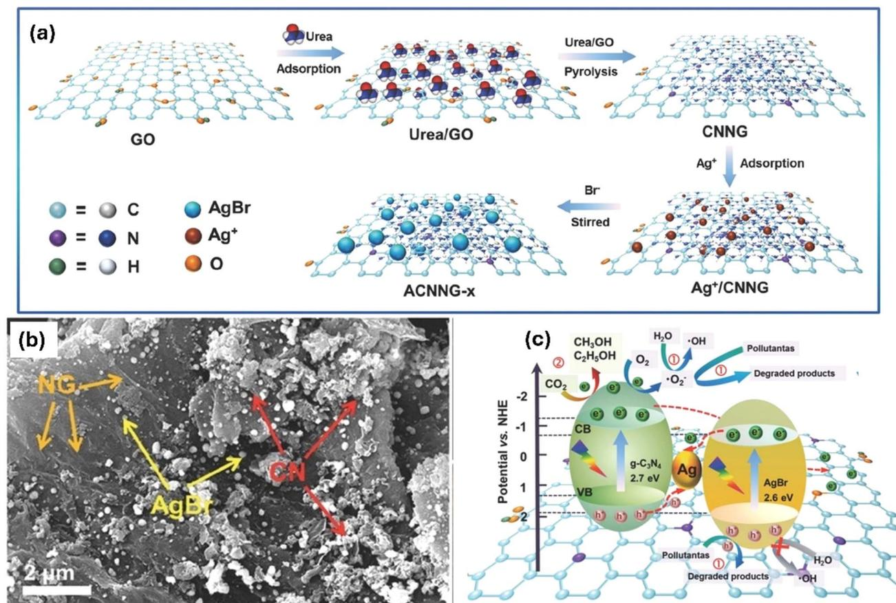
Fig. 14 (a) Synthesis process of ACNNG-x hybrid, and (b) its SEM image, and (c) a mechanism for CO<sub>2</sub> reduction by the hybrid nanocomposites, reprinted with the permission of ref. 264, copyright 2024, Elsevier.
