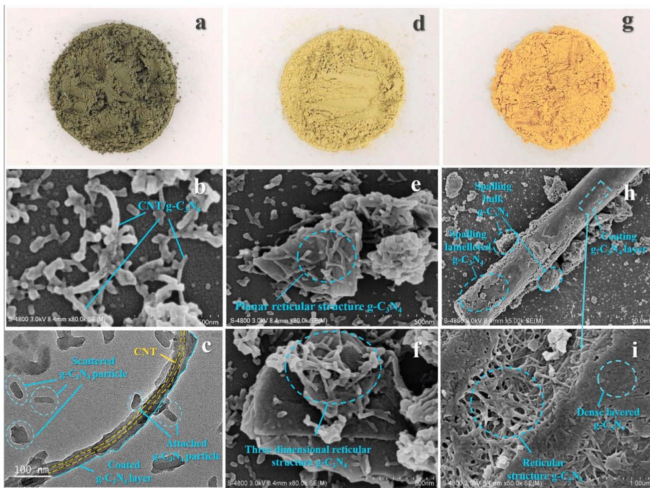
Fig. 7 Macro shots of (a–c) CNT/g-C<sub>3</sub>N<sub>4</sub>, GN/g-C<sub>3</sub>N<sub>4</sub> and CF/g-C<sub>3</sub>N<sub>4</sub>. SEM images of (d–f) CNT/g-C<sub>3</sub>N<sub>4</sub>, GN/g-C<sub>3</sub>N<sub>4</sub> and CF/g-C<sub>3</sub>N<sub>4</sub>. TEM images of (g–i) CNT/g-C<sub>3</sub>N<sub>4</sub>, GN/g-C<sub>3</sub>N<sub>4</sub> and CF/g-C<sub>3</sub>N<sub>4</sub>, reprinted with the permission of ref. 155, copyright 2024, Elsevier.
