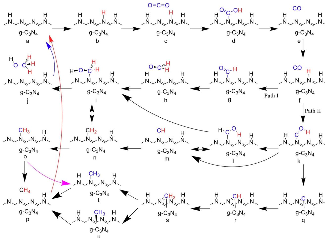
Fig. 13 Proposed reaction pathway for CO<sub>2</sub> reduction to methanol and methane on the surface of g-C<sub>3</sub>N<sub>4</sub>, reprinted with the permission of ref. 258, copyright 2024, Elsevier.
