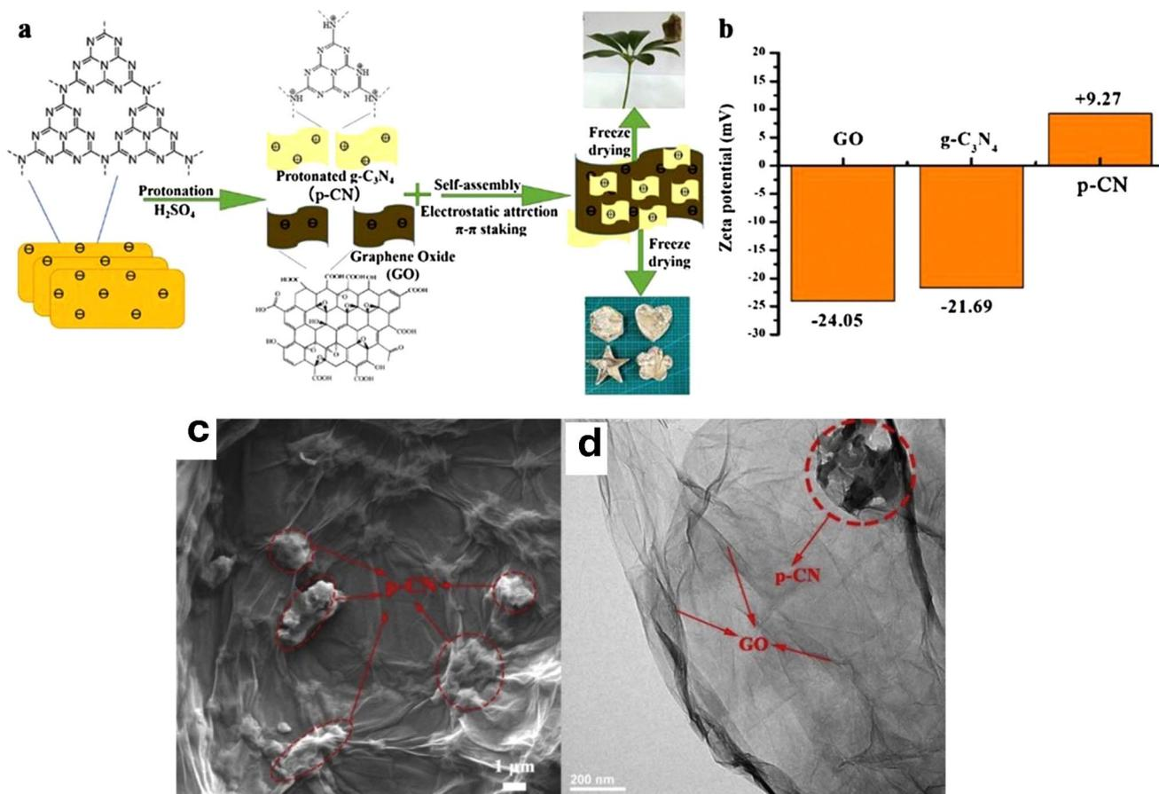
Fig. 6 (a) Schematic of the fabrication of p-CN/GOA; (b) zeta potential of GO,  $g\text{-C}_3\text{N}_4$  and p-CN, (c) the SEM of p-CN/GOA; (d) the TEM of p-CN/GOA, reprinted with the permission of ref. 152, copyright 2024, Elsevier.
