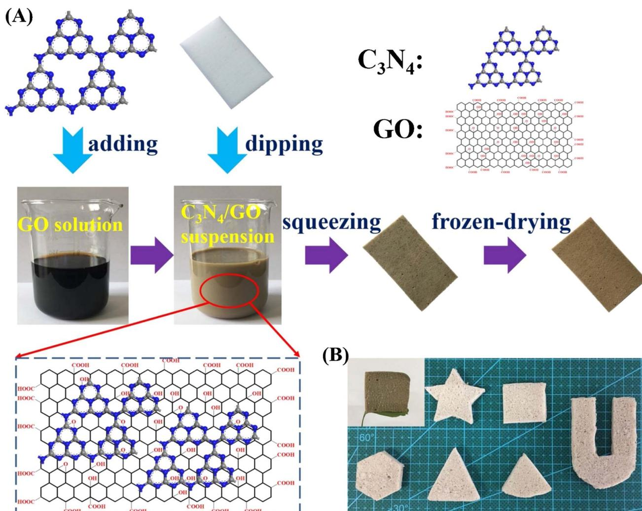
Fig. 5 (a) Schematic illustration of the preparation of  $\text{g-C}_3\text{N}_4/\text{GO}$ -wrapped sponge; (B): image of different shapes of  $\text{g-C}_3\text{N}_4/\text{GO}$ -wrapped sponge, reprinted with the permission of ref. 150, copyright 2024, Elsevier.
