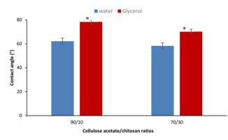
Fig. 1 Contact angle assessment of the different nanofiber scaffolds using water and glycerol as solvent tests. Data presented as mean  $\pm$  SD. Mean values followed by (\*) means that results are significantly different at p < 0.05.
