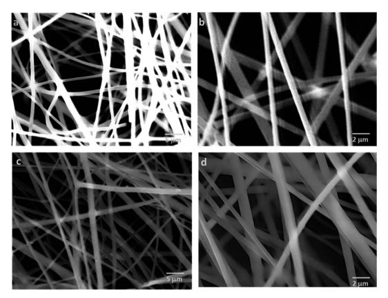
Fig. 2 SEM micrographs of MC/CTR/CS crosslinked nanofiber mats: (a) blend ratio 90/10, magnification  $5000 \times$ , (b) blend ratio 70/30,  $10000 \times$ , (c) blend ratio 70/30,  $5000 \times$ , (d) blend ratio 70/30,  $10000 \times$ .
