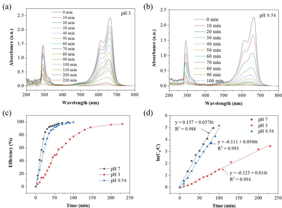
Fig. 10 The impact of solution pH on the photocatalytic activity of the ZnO : Fe<sub>2</sub>O<sub>3</sub> = 3 : 2 sample at (a) pH 3 and (b) pH 9.54; the dependence of the photocatalytic efficiency (c) and ln(C<sub>0</sub>/C) (d) on illumination time with an initial MB concentration of 10 ppm.
