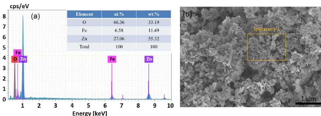
Fig. 4 (a) The energy-dispersive X-ray spectrum (EDS) of the ZnO : Fe<sub>2</sub>O<sub>3</sub> = 3 : 2 hybrid, and (b) the corresponding area of the SEM image.
