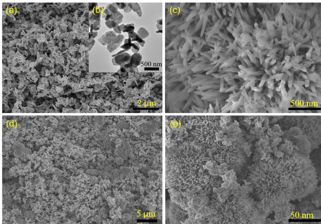
Fig. 3 (a) SEM image of ZnO, (b) TEM image of ZnO, (c) SEM image of Fe<sub>2</sub>O<sub>3</sub>, and SEM images of ZnO/Fe<sub>2</sub>O<sub>3</sub> with magnifications of (d) 2,000, and (e) 10 000.
