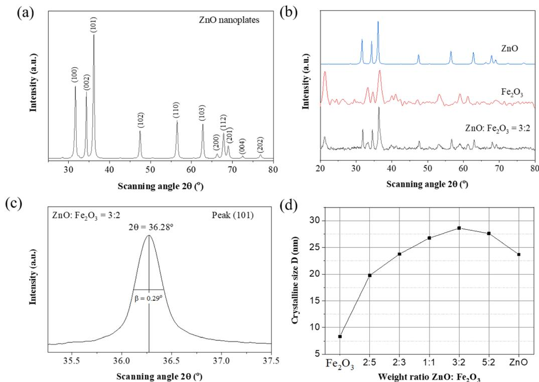
Fig. 2 (a) XRD patterns of ZnO nanoplates. (b) Comparison of the XRD patterns of pure ZnO, pristine  $\text{Fe}_2\text{O}_3$  nanospindles and ZnO/ $\text{Fe}_2\text{O}_3$  hybrids with a ZnO :  $\text{Fe}_2\text{O}_3$  weight ratio of 3 : 2. (c) The full width at half maximum of a diffraction peak and Bragg diffraction angle; (d) the dependence of crystallite size on the ZnO :  $\text{Fe}_2\text{O}_3$  weight ratio.
