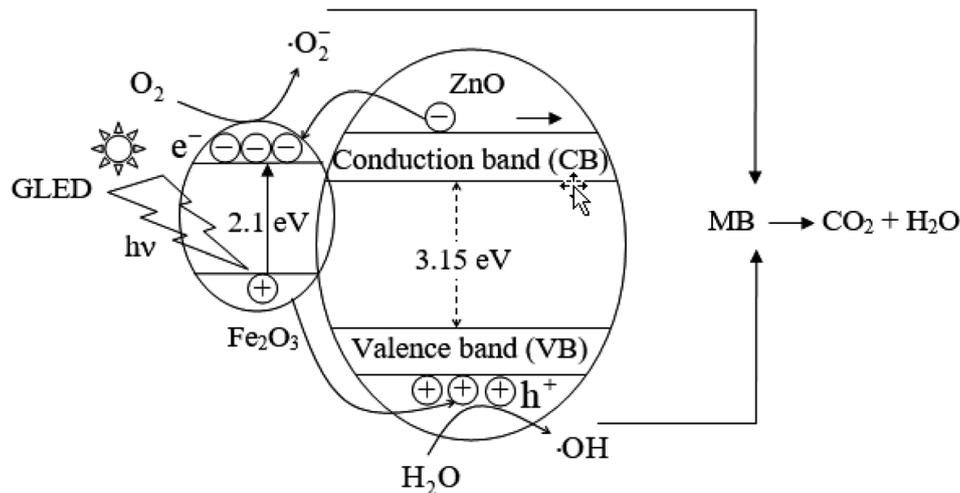
Fig. 12 A schematic diagram showing the role of the heterojunction of ZnO/Fe<sub>2</sub>O<sub>3</sub>.
