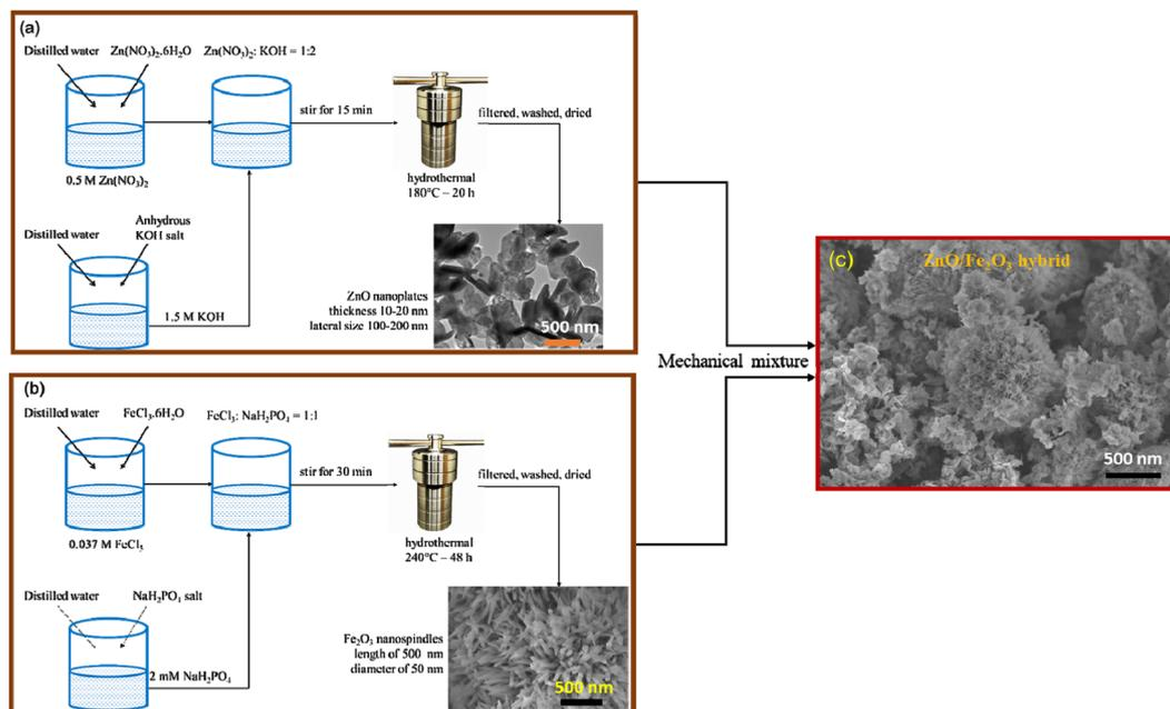
Fig. 1 Schematic of the preparation of (a) ZnO nanoplates, (b) Fe<sub>2</sub>O<sub>3</sub> nanospindles, and (c) ZnO/Fe<sub>2</sub>O<sub>3</sub> hybrid materials.
