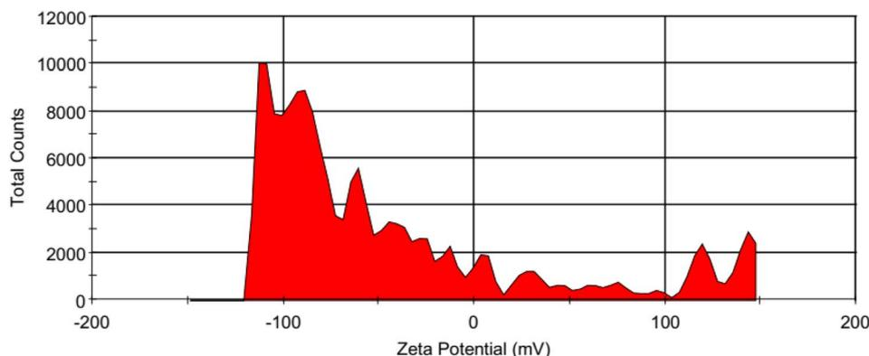
Fig. 6 Zeta potential distribution of the  $\text{ZnO}:\text{Fe}_2\text{O}_3 = 3:2$  sample.
