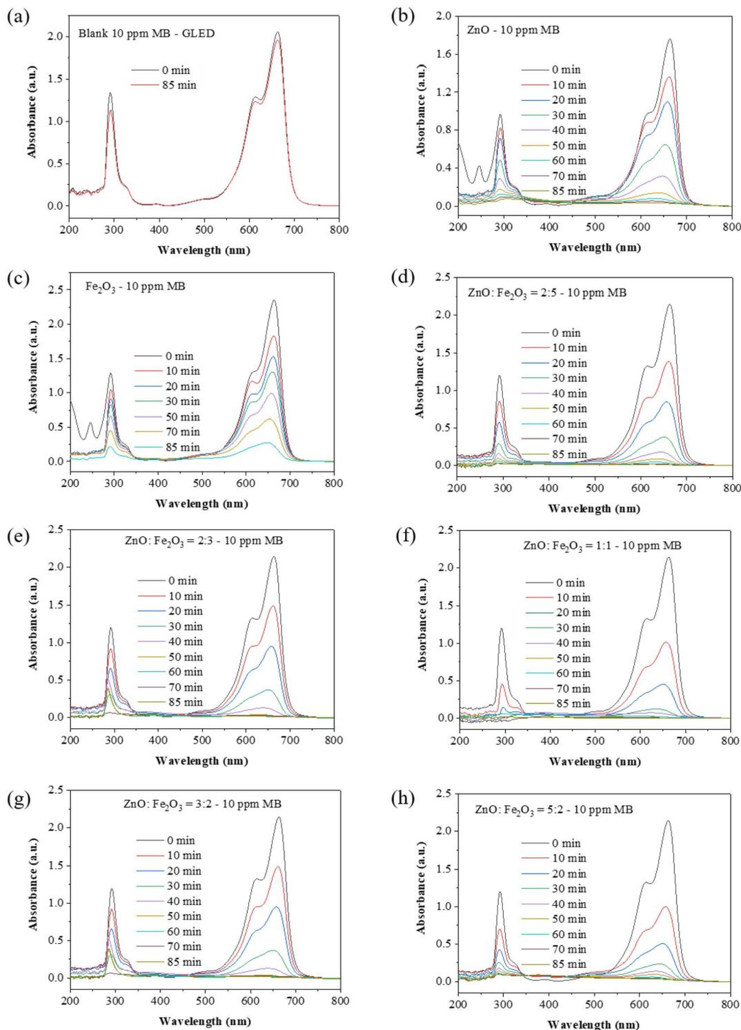
Fig. 7 UV-vis absorbance spectra of (a) the blank 10 ppm MB solution without a catalyst before and after GLED illumination for 85 min; (b) pure ZnO; (c) pristine  $\text{Fe}_2\text{O}_3$ ; and ZnO/ $\text{Fe}_2\text{O}_3$  with different ZnO :  $\text{Fe}_2\text{O}_3$  weight ratios of (d) 2 : 5, (e) 2 : 3, (f) 1 : 1, (g) 3 : 2, and (h) 5 : 2 under GLED illumination for 0–85 min.
