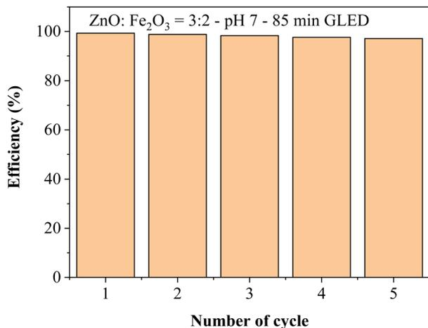
Fig. 11 The recyclability of the ZnO:Fe<sub>2</sub>O<sub>3</sub> = 3:2 sample at pH 7 towards 10 ppm MB after 5 cycles.
