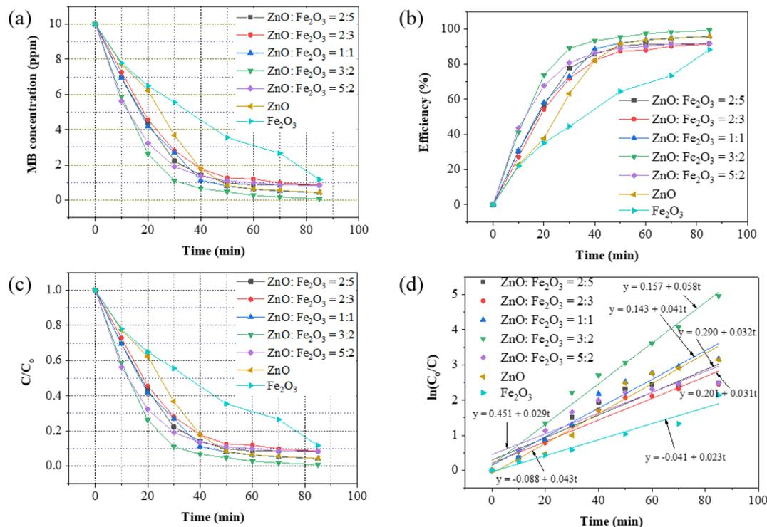
Fig. 8 (a) The dependence of MB concentration on the irradiation time of different samples, (b) the photocatalytic efficiency of different samples, (c) the dependence of  $C/C_0$  on irradiation time, and (d) the photocatalytic degradation rate of different samples.
