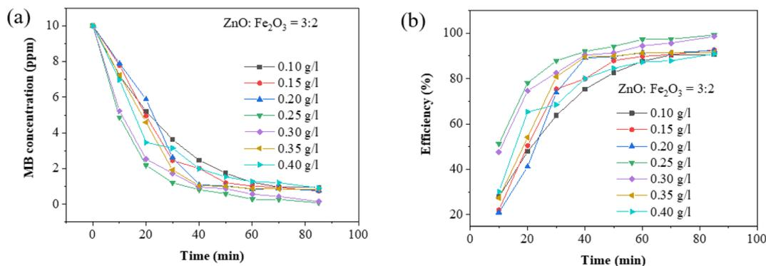
Fig. 9 (a) The dependence of MB concentration on the irradiation times of different amounts of the ZnO : Fe<sub>2</sub>O<sub>3</sub> = 3 : 2 sample; (b) a comparison of the photocatalytic efficiencies of different amounts of the ZnO : Fe<sub>2</sub>O<sub>3</sub> = 3 : 2 sample.
