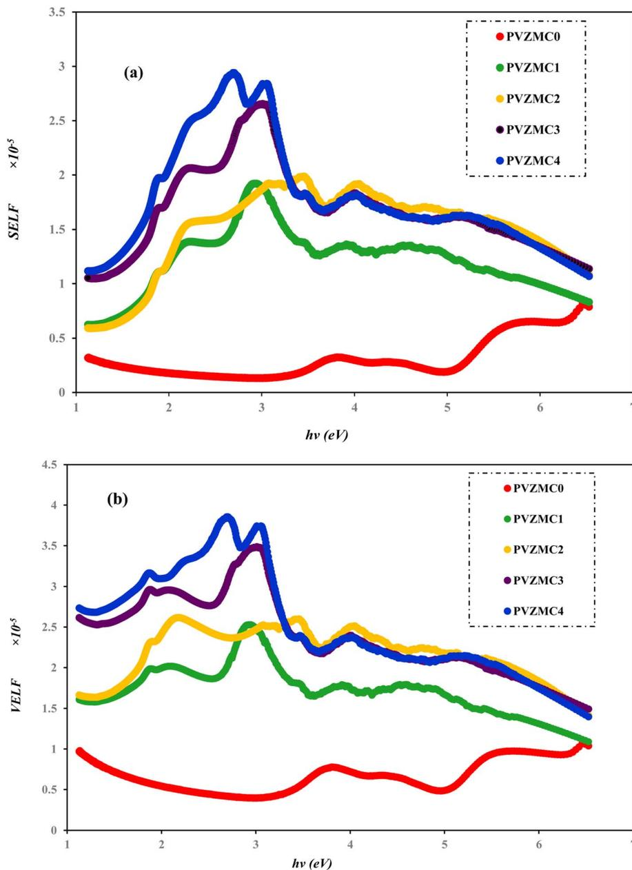
Fig. 19 (a) SELF and (b) VELF vs. photon energy functions for the PVA and PVA/Zn-metal complex films.
