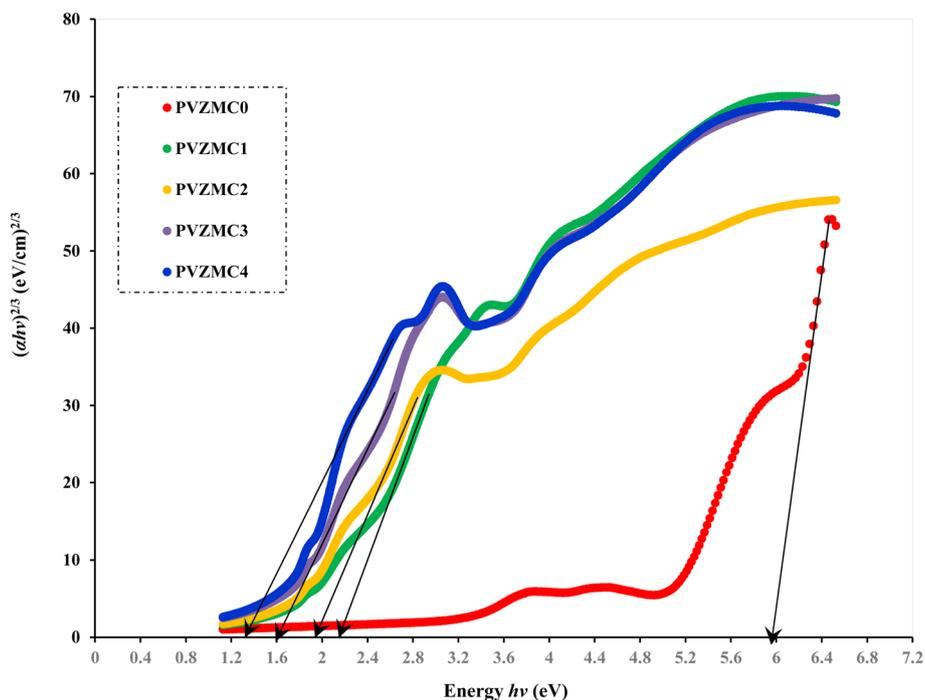
Fig. 10 Direct forbidden band gap energy plot of pure polymer PVA and composite PVA/Zn-metal complex films.
