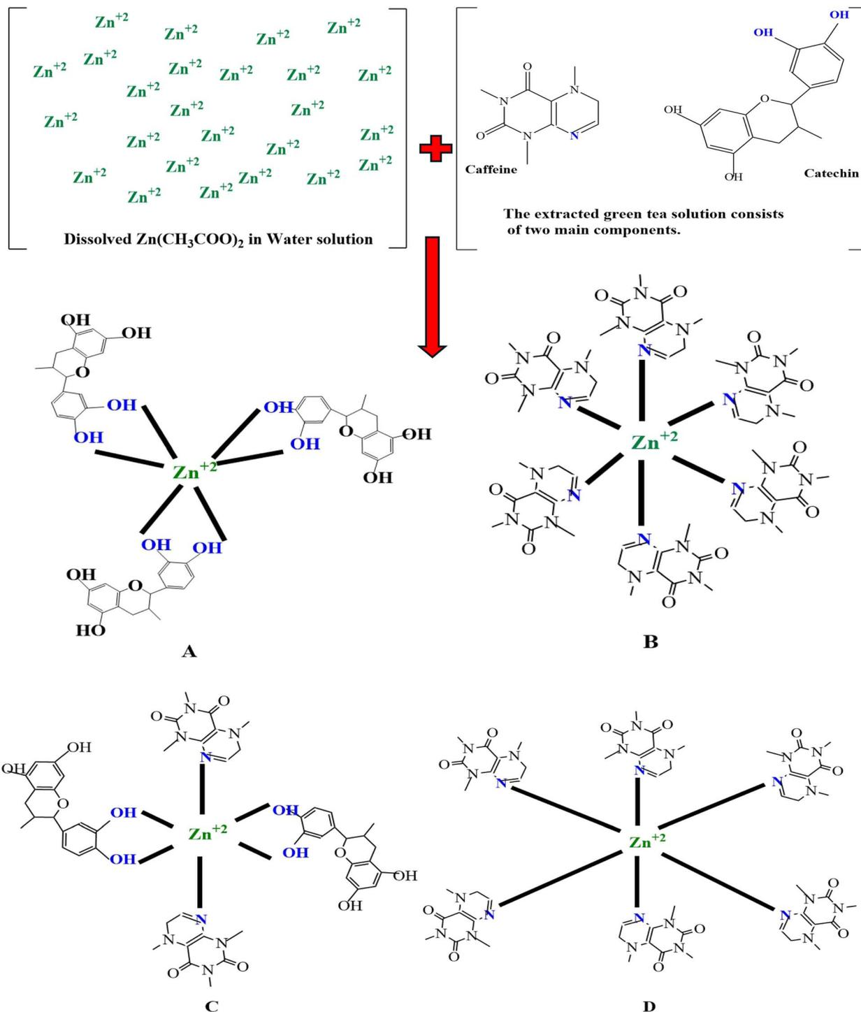
**Scheme 4** The proposed structure for producing metal complexes involves binding ligands Caffeine and catechin to central metal ions,  $Zn^{2+}$ . The compounds mentioned are (A) a bidentate complex of  $[Zn(C_{15}H_{14}O_6)_3]$ , (B) a monodentate complex of  $[Zn(C_8H_{10}N_4O_2)_6]$ , (C) a complex with both bidentate and monodentate  $[Zn(C_{15}H_{14}O_6)_2(C_8H_{10}N_4O_2)_2]$ , and (D) monodentate  $[Zn(C_8H_{10}N_4O_2)_6]$  structure.
