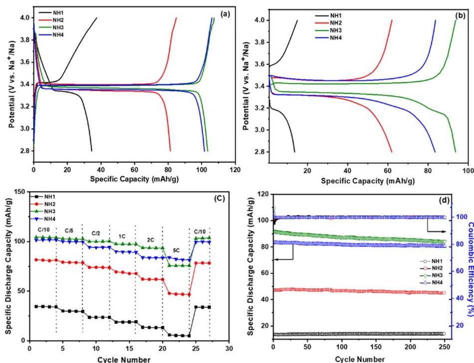
Fig. 4 (a) The first charge–discharge profiles at 0.1C (b) first charge–discharge profiles at 1C, (c) rate capability of NVP@C at different temperatures in a potential range of 2.8–4.0 V vs. Na/Na<sup>+</sup>, (d) cyclability at a rate of 2C.
