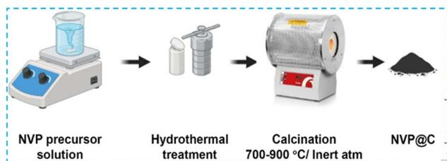
Scheme 1 Synthesis process of the Na<sub>3</sub>V<sub>2</sub>(PO<sub>4</sub>)<sub>3</sub>@C samples.
