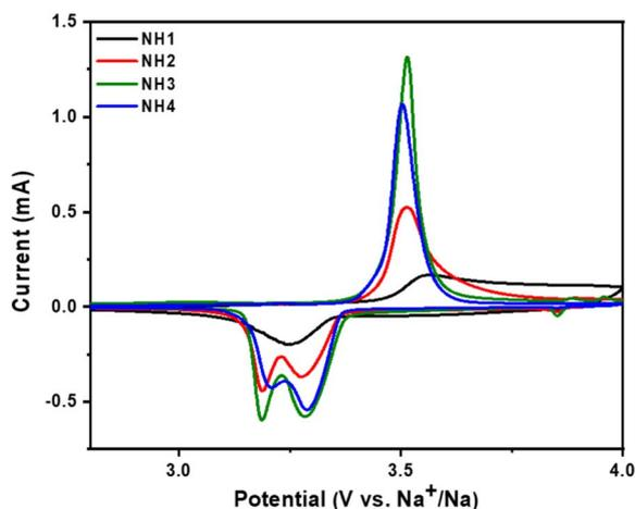
Fig. 3 1st Cyclic voltammetry (CV) curves of the NVP@C cycled between 2.8 and 4.0 V at a scan rate of 0.1 mV s<sup>-1</sup> calcined at different temperatures.
