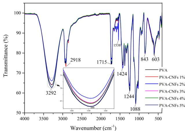
Fig. 4 The FTIR of PVA and bio-nanocomposite films.
