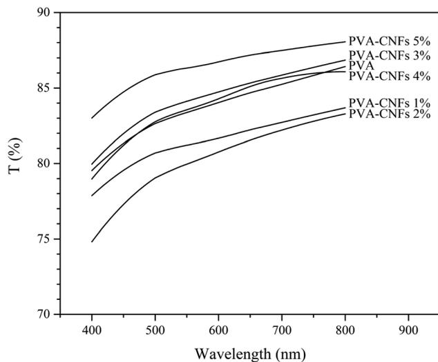
Fig. 3 The UV-VIS of PVA and bio-nanocomposite films.
