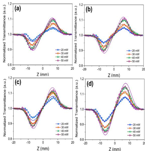
Fig. 6 CA curves of (a) VSe<sub>2</sub> pure, (b) 5%, (c) 10%, and (d) 20% Co precursor in VSe<sub>2</sub>-CoSe<sub>2</sub> nanostructures, at different incident power of the laser.
