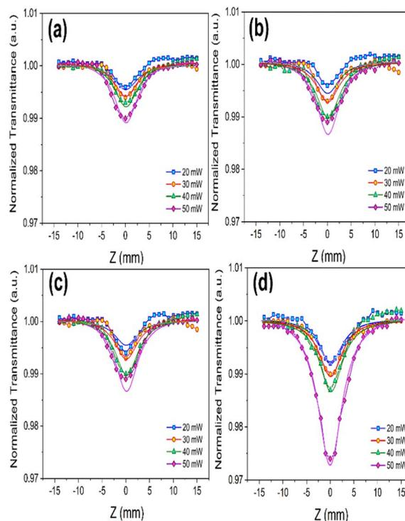
Fig. 5 OA curves of (a) Pure VSe<sub>2</sub>, (b) 5%, (c) 10%, and (d) 20% Co of VSe<sub>2</sub>-CoSe<sub>2</sub> nanostructures, at different incident power of the laser.
