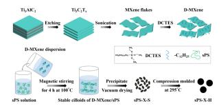
**Scheme 1** The preparation process of MXene, p-MXene and p-MXene/sPS nanocomposites.
