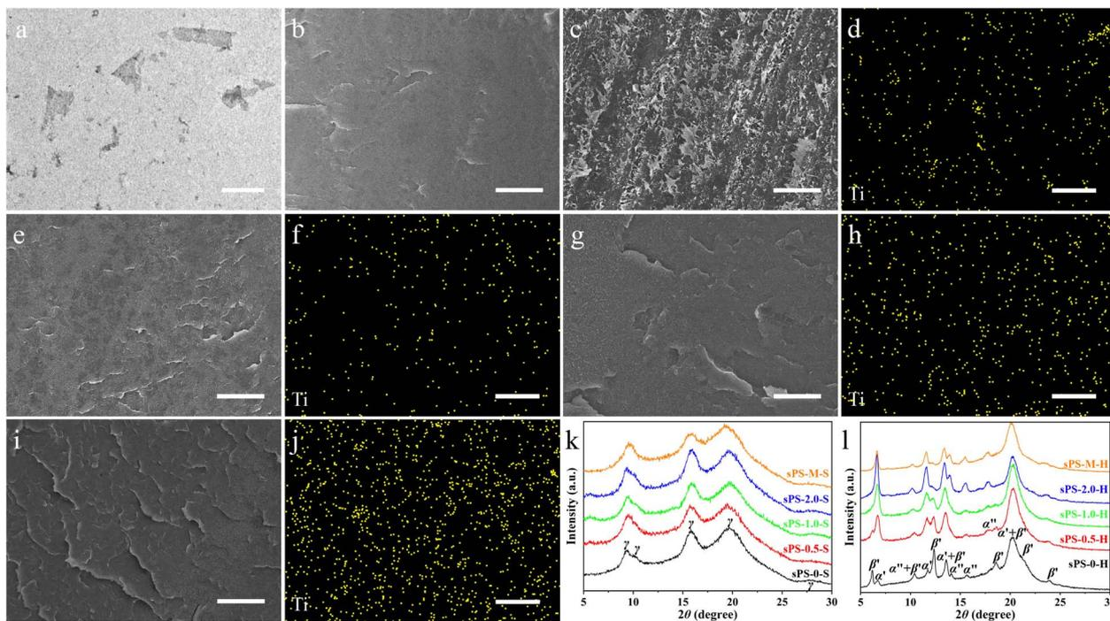
Fig. 2 TEM image of (a) sPS-2.0-S, the scale bar is 1  $\mu\text{m}$ . SEM images of cross-section of (b) sPS-0-H, (c) sPS-M-H, (e) sPS-0.5-H, (g) sPS-1.0-H, and (i) sPS-2.0-H after brittle fracture, EDX mappings of Ti for (d) sPS-M-H, (f) sPS-0.5-H, (h) sPS-1.0-H, and (j) sPS-2.0-H, the scale bars are 10  $\mu\text{m}$ . Conventional XRD patterns of (k) sPS-X-S, and (l) sPS-X-H.
