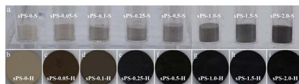
Fig. 1 (a) Photographs of solution mixed  $\text{D-MXene/sPS}$  nanocomposites with different  $\text{D-MXene}$  concentrations. (b–i) Photographs of hot-pressed  $\text{D-MXene/sPS}$  nanocomposites with different  $\text{D-MXene}$  concentrations after solution mixed.
