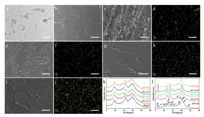
Fig. 2 TEM image of (a) sPS-2.0-S, the scale bar is 1  $\mu$ m. SEM images of cross-section of (b) sPS-0-H, (c) sPS-M-H, (e) sPS-0.5-H, (g) sPS-1.0-H, and (i) sPS-2.0-H after brittle fracture, EDX mappings of Ti for (d) sPS-M-H, (f) sPS-0.5-H, (h) sPS-1.0-H, and (j) sPS-2.0-H, the scale bars are 10  $\mu$ m. Conventional XRD patterns of (k) sPS-X-S, and (l) sPS-X-H.
