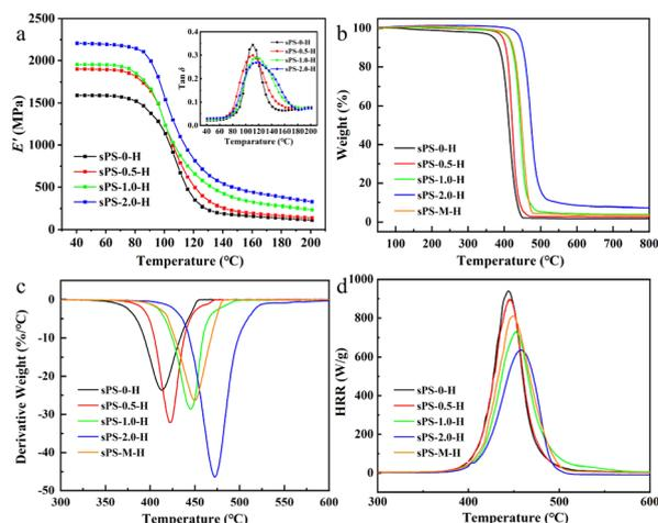
Fig. 5 (a) Temperature dependence of  $E'$  and  $\tan \delta$  (inset), (b) TG, (c) DTG, and (d) MCC curves of neat sPS and sPS nanocomposites.
