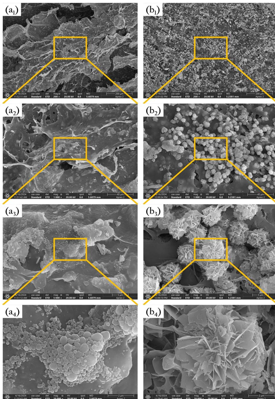
Fig. 5 SEM images of OSP@Gel: (a) before phosphate adsorption; (b) after phosphate adsorption.
