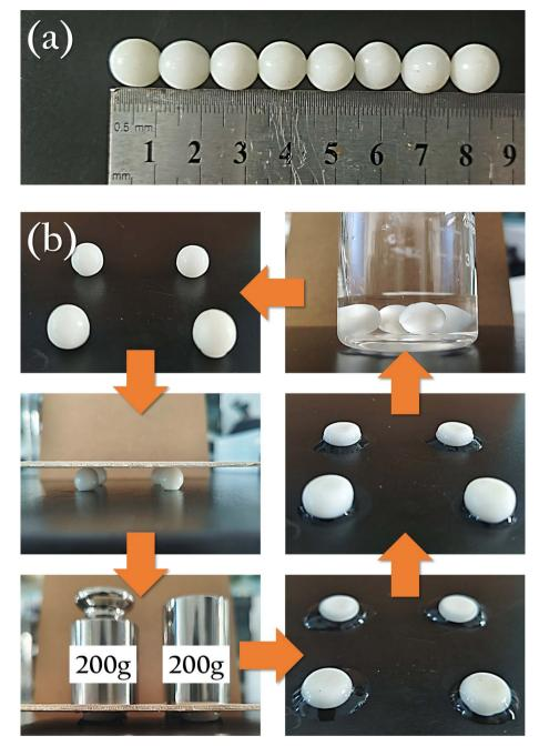
Fig. 4 (a) Optical images of OSP@Gel beads; (b) compression and recovery of OSP@Gel beads.
