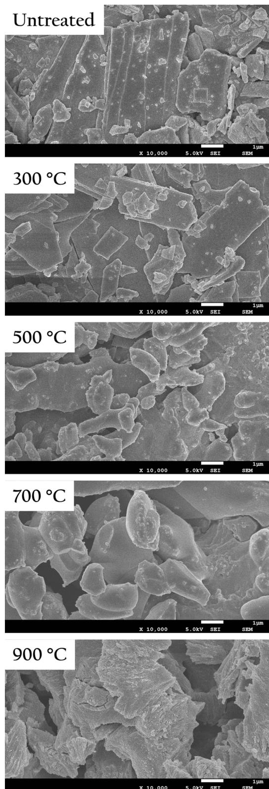
Fig. 1 SEM images of OSP under different thermal treatment temperatures.
