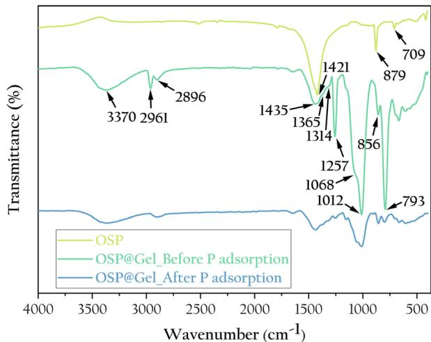
Fig. 6 FTIR spectra of the OSP, OSP@Gel before and after phosphate adsorption.
