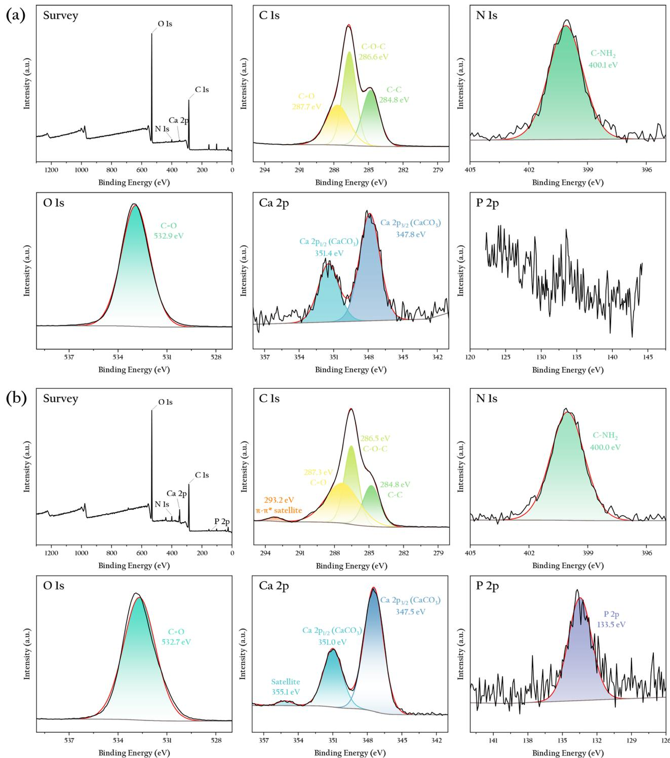
Fig. 7 XPS spectra of the OSP@Gel sample: (a) before phosphate adsorption; (b) after phosphate adsorption.
