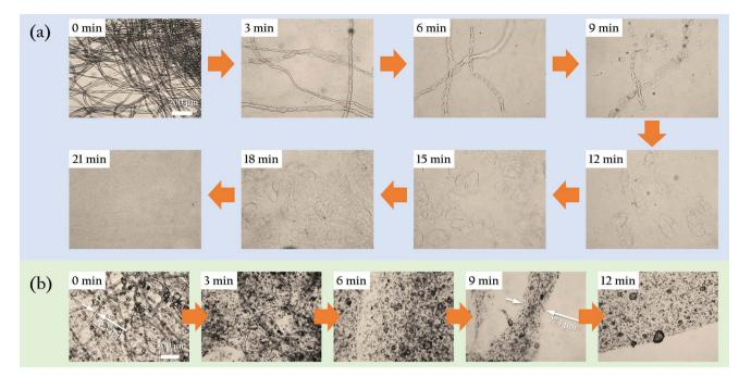
Fig. 3 Optical microscopic images of the fiber gelation process: (a) without OSP; (b) with OSP
