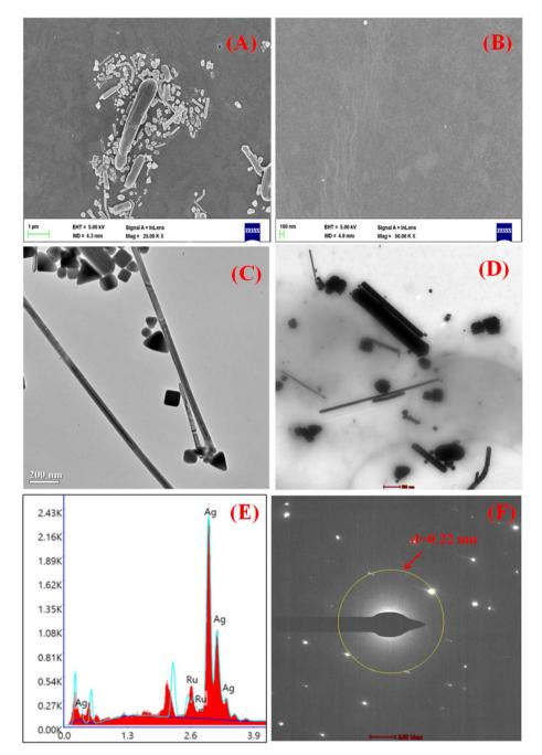
Fig. 5 (A and B) SEM image of LB composite film in  $\mu$ m and nm scale, (C and D) TEM image of AgNWs with and without pesticide interaction, (E and F) EDX and SAED pattern analysis, respectively.
