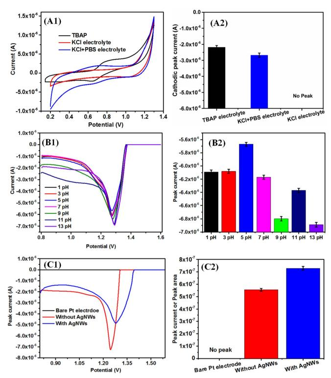
Fig. 6 (A1) CV graph of Pt modified electrode using different electrolytes (A2) bar diagram for the different electrolyte *versus* current, (B1) DPV variation of the different pH (1–11), (B2) bar diagram for the different pH  $\nu$  versus current (10  $\mu$ M). (C1) DPV variation of Pt modified electrode in the presence of AgNWs, (C2) Bar diagram for the presence of AgNWs on Pt modified electrode  $\nu$  current.
