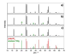
Fig. 2 XRD patterns of (a) UCPs (β-NaYF4:Yb³+,Tm³+) crystals, (b) UCPs + P25 (β-NaYF4:Yb³+,Tm³+ mixed with P25) sample and (c) UCPs@TiO $_2$  (β-NaYF $_4$ :Yb³+,Tm³+ coated with TiO $_2$ ) sample. "A" indicates reflections characteristic for TiO $_2$  anatase.
