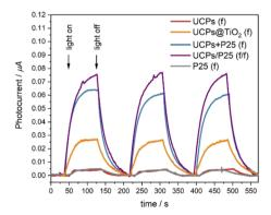
Fig. 4 Photocurrent response of UCPs, UCPs coated with titania (UCPs@TiO $_2$ (f)), UCPs mixed with P25 (UCPs + P25(f)), spatially separated UCPs and P25 deposited on two different ITO foil pieces (UCPs/P25(f/f)) and P25 under 980 nm excitation.
