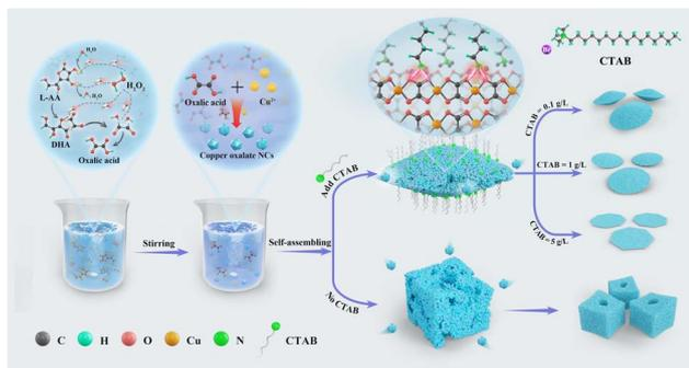
Fig. 8 Schematic diagram of copper oxalate precipitation. Effect of CTAB on the assembly process of copper oxalate nanocrystals.
