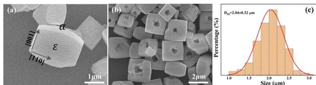
**Fig. 1** (a) Typical SEM morphology of copper oxalate crystals obtained based upon the conventional synthesis method; (b) SEM image of copper oxalate crystals prepared using L-ascorbic acid acting as a source of oxalate ligand without the addition of CTAB; (c) histogram of lateral dimensions of copper oxalate crystals in (b).
