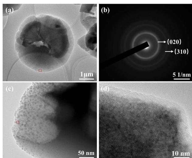
Fig. 4 Typical TEM morphology of (a) copper oxalate crystals at CTAB addition of  $1 \text{ g L}^{-1}$ ; (b) selected electron diffraction pattern of the red-marked part in (a); (c) localized TEM image of copper oxalate crystals; (d) HRTEM image of the red-marked part in (c).
