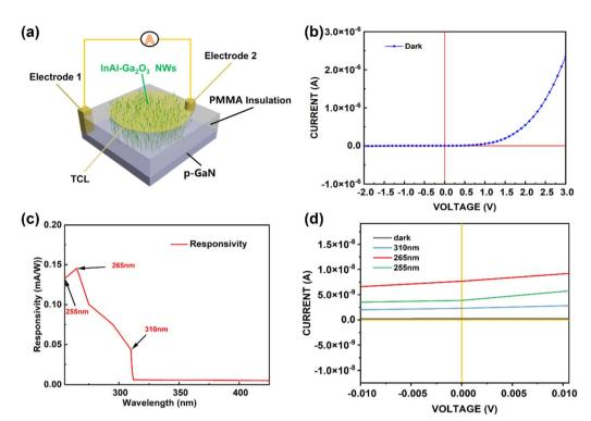
Fig. 3 The structure and characteristics of GaN/InAl-Ga<sub>2</sub>O<sub>3</sub> NWs UVPD. (a) Structure diagram of GaN/InAl-Ga<sub>2</sub>O<sub>3</sub> NWs UVPD. (b) GaN/InAl-Ga<sub>2</sub>O<sub>3</sub> NWs UVPD. (c) Spectral response curve of GaN/InAl-Ga<sub>2</sub>O<sub>3</sub> NWs UVPD. (d) I-V characteristic amplification curves of near zero bias for 255 nm, 265 nm and 310 nm light sources.
