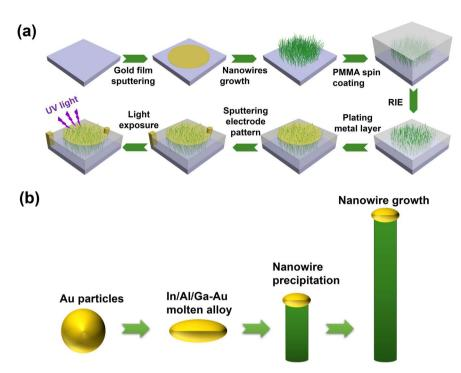
Process schematic diagram. (a) Preparation process flow chart. (b) Schematic diagram of InAl-Ga<sub>2</sub>O<sub>3</sub> NWs growth principle.
