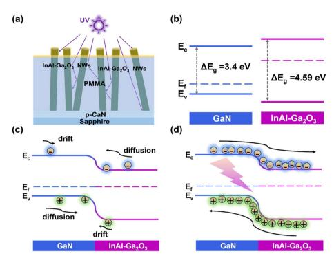
Fig. 5 Band configuration analysis. (a) Schematic diagram of device cross-section structure. (b) GaN and InAl-Ga<sub>2</sub>O<sub>3</sub> NWs band alignment before contact. Post-contact: (c)  $GaN/InAl-Ga_2O_3p-n$  junction band arrangement in dark environment; (d) band map under zero-bias under UV irradiation.
