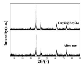
Fig. 8 XRD patterns of Cu<sub>2</sub>O@Fe<sub>3</sub>O<sub>4</sub> contrast after five cycling reactions.
