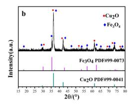
Fig. 1 (a) XRD patterns of Fe<sub>3</sub>O<sub>4</sub> and (b) Cu<sub>2</sub>O@Fe<sub>3</sub>O<sub>4</sub>.
