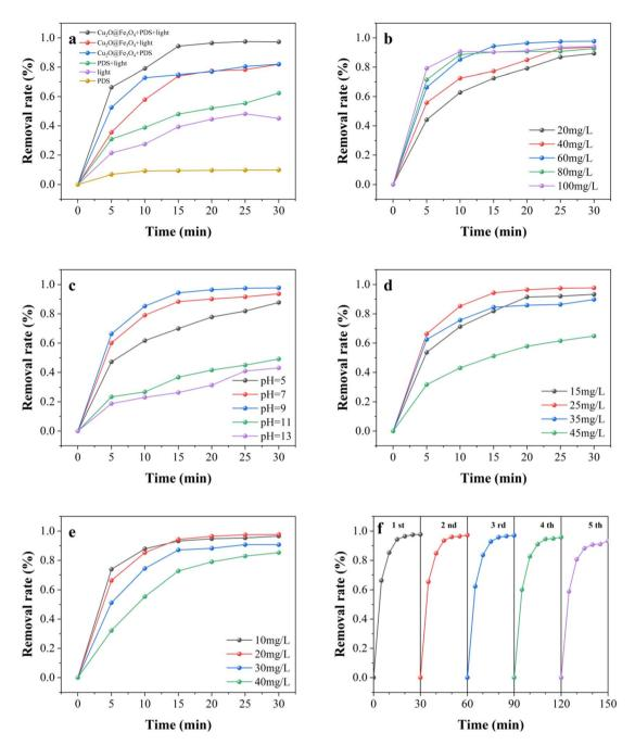
Fig. 7 (a) Comparison of the different reaction systems; (b) effect of  $Cu_2O@Fe_3O_4$  dosage on TC removal performance; (c) effect of pH on TC removal performance; (d) effect of PDS dosage on TC removal performance; (e) effect of the initial TC concentration on TC removal performance; (f) recyclability and stability of the catalyst.
