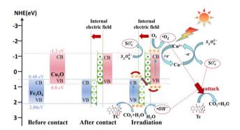
Fig. 11  $Cu_2O@Fe_3O_4$  mechanism of removal of TC by photocatalytic activation of PDS.
