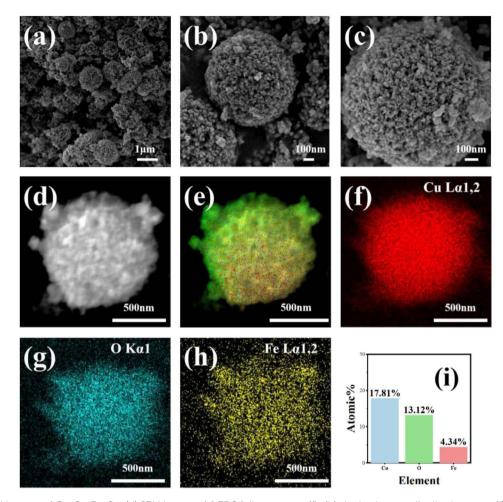
Fig. 3 (a)–(c) SEM images of  $Cu_2O@Fe_3O_4$ ; (d) SEM images; (e) EDS full spectrum; (f)–(h) single element distribution map: (f) Cu; (g) Fe; (h) O; (i) the atomic content of Cu, O, and Fe.
