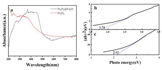
Fig. 5 (a) UV-Vis diffuse reflectance spectra of  $Cu_2O@Fe_3O_4$  and  $Fe_3O_4$ , (b)  $(\alpha h\nu)^2$  and  $h\nu$  curves of  $Fe_3O_4@Cu_2O$  samples, (c)  $(\alpha h\nu)^2$  and  $h\nu$  curves of  $Fe_3O_4$  samples.
