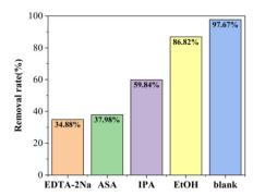
Fig. 10 Degradation of TC by  $Cu_2O@Fe_3O_4$  composite catalyst in different free radical scavengers.
