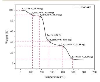
Fig. 3 TGA thermogram of synthesized PVC-g-AEP polymer.
