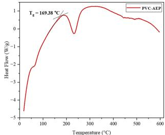
DSC thermogram of synthesized polymer.
