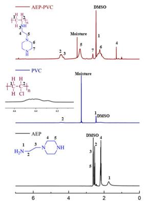
Fig. 2 <sup>1</sup>H-NMR spectra of synthesized polymer, PVC, and AEP.
