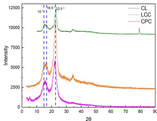
Fig. 6 X-ray diffractogram of CL, LCC, and CPC.
