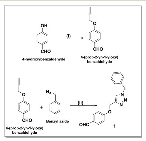
Scheme 1 Synthesis of the 4-[(1-benzyl-1H-1,2,3-triazol-4-yl)methoxylbenzaldehyde (a) reaction conditions: (i) propargyl bromide, acetone,  $K_2CO_3$ , 2 h. (ii)  $CuSO_4$ , sodium ascorbate, DMF/water (8 : 2), 3 h.
