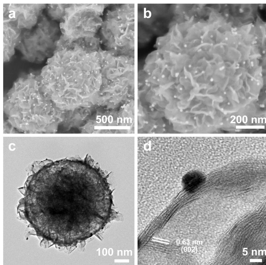
Fig. 1 SEM images at different magnifications of the yolk-shell Au@MoS<sub>2</sub> (a and b). TEM images at different magnifications of yolk-shell Au@MoS<sub>2</sub> (c and d). SEM: scanning electron microscope. TEM: transmission electron microscopy.
