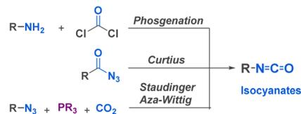
Fig. 2 Several examples of reactions producing isocyanates.
