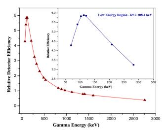
Fig. 5 In situ relative detector efficiency calibration.
