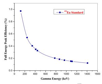
Fig. 4 Full energy peak efficiency calibration using <sup>152</sup>Eu standard.
