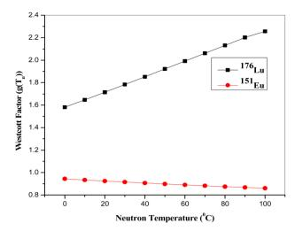
Fig. 7 Westcott factor for the non-1/v nuclides using ENDF/B-VIII.0 data (USA, 2018).
