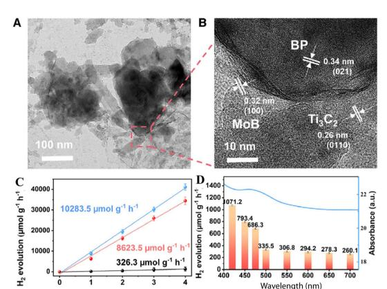
Fig. 12 (A) TEM image, (B) HRTEM image, (C) hydrogen production (red line =  $\lambda \ge 420$  nm; blue line = full spectrum; black line = near IR) and (D) wavelength-dependent photocatalytic hydrogen production of the black phosphorous/Ti<sub>3</sub>C<sub>2</sub>/MBene tertiary nanocomposite. This figure has been reproduced from ref. 78 with permission from Elsevier, Copyright 2024.
