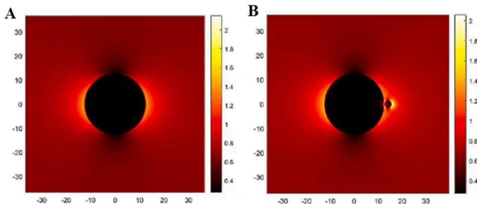
Fig. 6 Electric field distribution calculated from FDTD simulations for (A)  $\text{TiO}_2$  and (B)  $\text{CDs/TiO}_2$ . The electric field's direction was polarised along the X-axis before incidentally intersecting the Z-axis. This figure has been reproduced from ref. 56 with permission from Elsevier, Copyright 2023.
