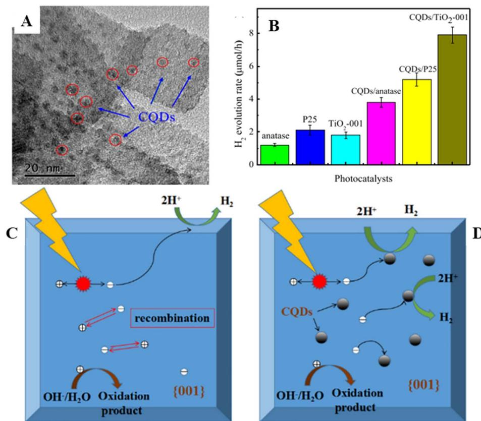
Fig. 5 (A) HRTEM image of CQDs/TiO<sub>2</sub>-001. (B) Photocatalytic hydrogen production of different photocatalysts based on TiO<sub>2</sub>-001. Illustration of charge transfer mechanisms and hydrogen production of (C) TiO<sub>2</sub>-001 and (D) CQDs/TiO<sub>2</sub>-001. This figure has been reproduced from ref. 51 with permission from Elsevier, Copyright 2019.
