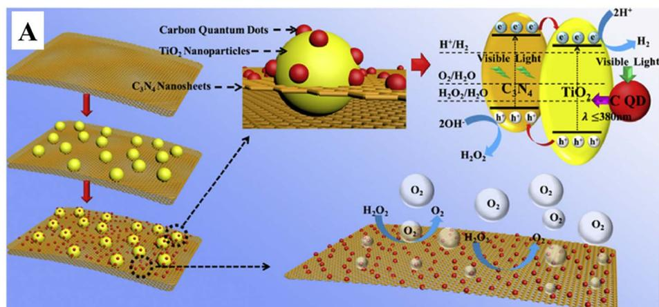
Fig. 11 (A) Schematic of the photocatalytic hydrogen production activity of the CQD-TiO<sub>2</sub>-C<sub>3</sub>N<sub>4</sub> tertiary composite. This figure has been reproduced from ref. 75 with permission from Elsevier, Copyright 2018.
