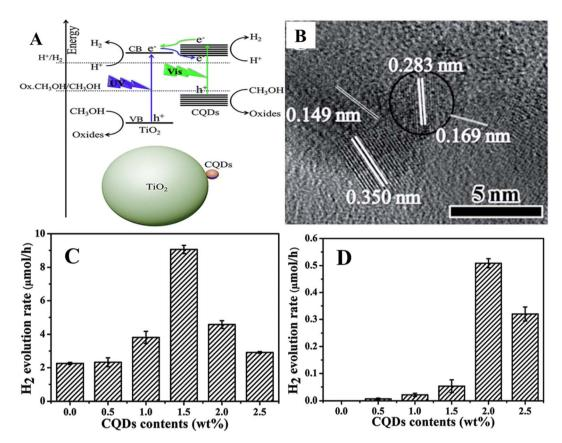
Fig. 3 (A) Schematic of the production of photocatalytic hydrogen using semiconductor ( $TiO_2$ )/CQDs when exposed to ultraviolet and visible light. (B) HRTEM image of CQD/ $TiO_2$  nanoparticles, and photocatalytic hydrogen production of CQDs/ $TiO_2$  under (C) UV-visible light and (D) visible light ( $\lambda \ge 450$  nm) irradiation. This figure has been reproduced from ref. 50 with permission from the Royal Society of Chemistry, Copyright 2014.
