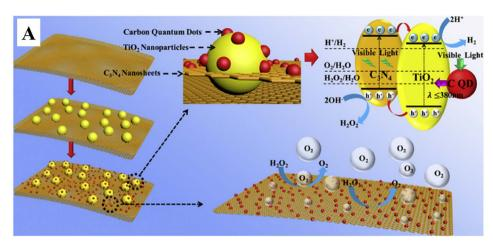
Fig. 11 (A) Schematic of the photocatalytic hydrogen production activity of the CQD-TiO<sub>2</sub>-C<sub>3</sub>N<sub>4</sub> tertiary composite. This figure has been reproduced from ref. 75 with permission from Elsevier, Copyright 2018.
