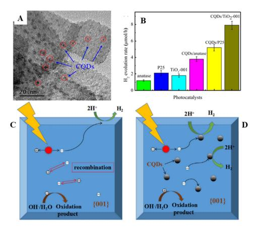
Fig. 5 (A) HRTEM image of CQDs/TiO $_2$ -001. (B) Photocatalytic hydrogen production of different photocatalysts based on TiO $_2$ -001. Illustration of charge transfer mechanisms and hydrogen production of (C) TiO $_2$ -001 and (D) CQDs/TiO $_2$ -001. This figure has been reproduced from ref. 51 with permission from Elsevier, Copyright 2019.
