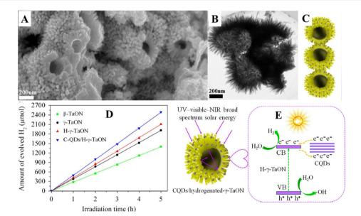
Fig. 8 (A) FESEM image, (B) TEM image, (C) schematic illustration, (D) photocatalytic hydrogen production and (E) schematic photocatalytic mechanism of CQD/γ-TaON heterojunctions. This figure has been reproduced from ref. 69 with permission from Elsevier, Copyright 2015.
