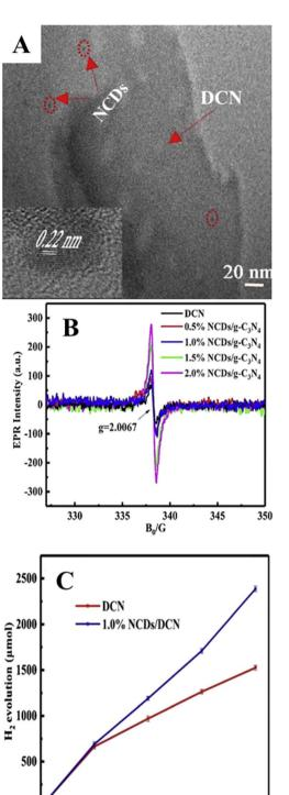
Fig. 10 (A) TEM image of 1% CQDs/graphitic carbon nitride (inset shows its lattice spacing). (B) electron spin resonance of CQDs/graphitic carbon nitride, (C) hydrogen evolution of 1% CQDs/graphitic carbon nitride. This figure has been reproduced from ref. 74 with the permission from Elsevier, Copyright 2020.
