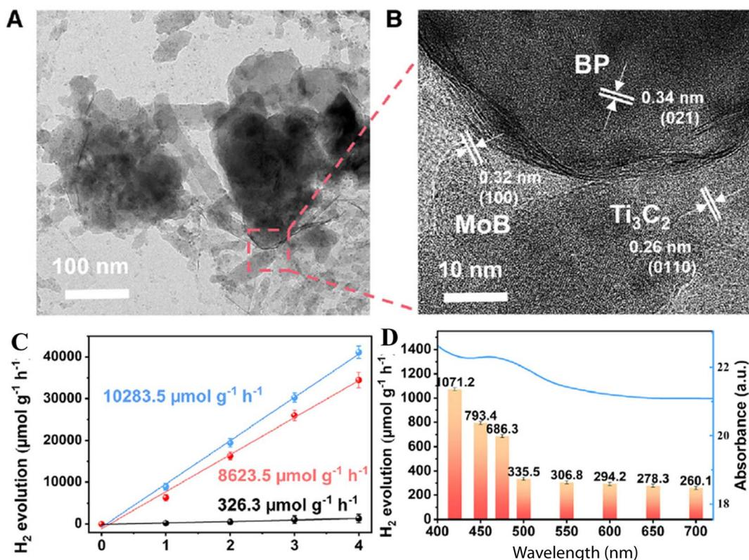
Fig. 12 (A) TEM image, (B) HRTEM image, (C) hydrogen production (red line =  $\lambda \geq 420 \text{ nm}$ ; blue line = full spectrum; black line = near IR) and (D) wavelength-dependent photocatalytic hydrogen production of the black phosphorus/ $\text{Ti}_3\text{C}_2$ /MBene tertiary nanocomposite. This figure has been reproduced from ref. 78 with permission from Elsevier, Copyright 2024.
