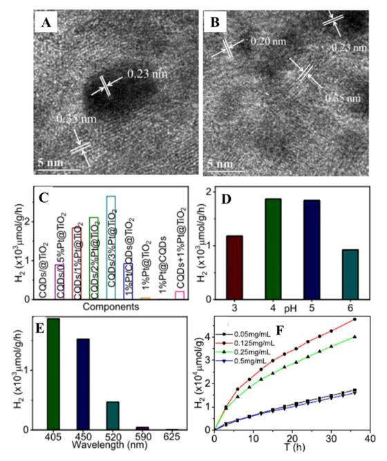
Fig. 4 (A and B) HRTEM images of CQDs/3 wt%Pt/TiO<sub>2</sub>. Hydrogen production dependence on (C) photocatalysts, (D) pH, (E) illuminated wavelength and (F) concentration of photocatalyst for CQD/1 wt%Pt/TiO<sub>2</sub> nanohybrids. This figure has been reproduced from ref. 54 with permission from the American Chemical Society, Copyright 2019.
