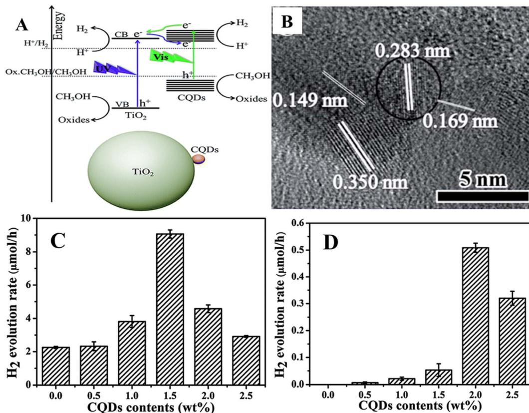
Fig. 3 (A) Schematic of the production of photocatalytic hydrogen using semiconductor (TiO<sub>2</sub>)/CQDs when exposed to ultraviolet and visible light. (B) HRTEM image of CQD/TiO<sub>2</sub> nanoparticles, and photocatalytic hydrogen production of CQDs/TiO<sub>2</sub> under (C) UV-visible light and (D) visible light ( $\lambda \geq 450$  nm) irradiation. This figure has been reproduced from ref. 50 with permission from the Royal Society of Chemistry, Copyright 2014.
