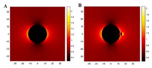
Fig. 6 Electric field distribution calculated from FDTD simulations for (A) TiO<sub>2</sub> and (B) CDs/TiO<sub>2</sub>. The electric field's direction was polarised along the X-axis before incidentally intersecting the Z-axis. This figure has been reproduced from ref. 56 with permission from Elsevier, Copyright 2023.
