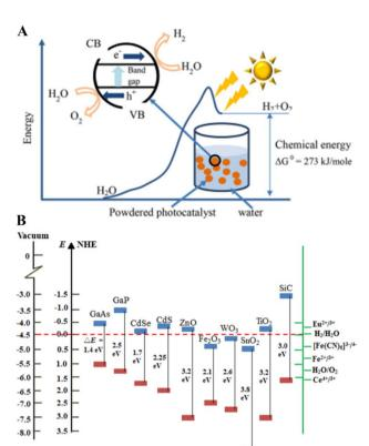
Fig. 2 (A) Schematic of the energy diagram of photocatalytic water splitting. (B) Energy band levels of different semiconductors. Inset in (A) shows the principle of photocatalytic water splitting. This figure has been reproduced from ref. 30 with permission from the Institute of Physics, Copyright 2021.
