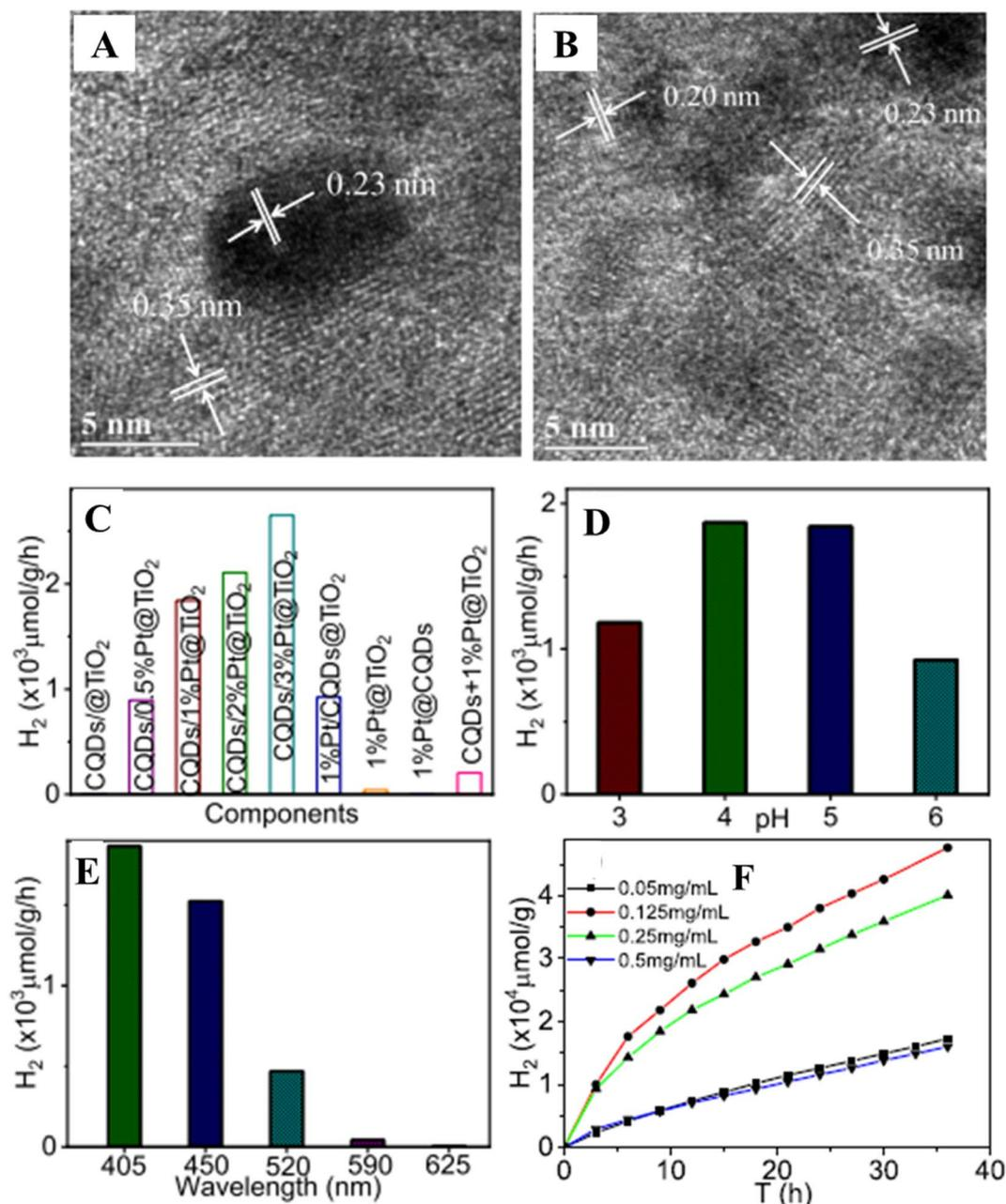
Fig. 4 (A and B) HRTEM images of CQDs/3 wt%Pt/TiO<sub>2</sub>. Hydrogen production dependence on (C) photocatalysts, (D) pH, (E) illuminated wavelength and (F) concentration of photocatalyst for CQD/1 wt%Pt/TiO<sub>2</sub> nanohybrids. This figure has been reproduced from ref. 54 with permission from the American Chemical Society, Copyright 2019.
