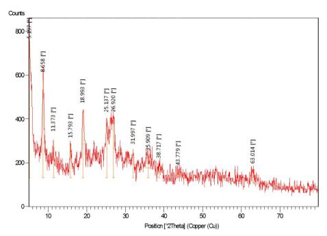
Fig. 5 The XRD spectrum of NGFRNH.
