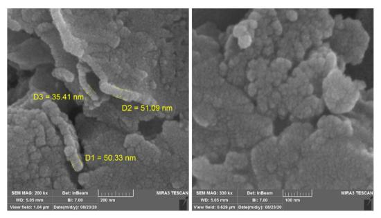
Fig. 3 The FE-SEM pictures of the nanocomposite.
