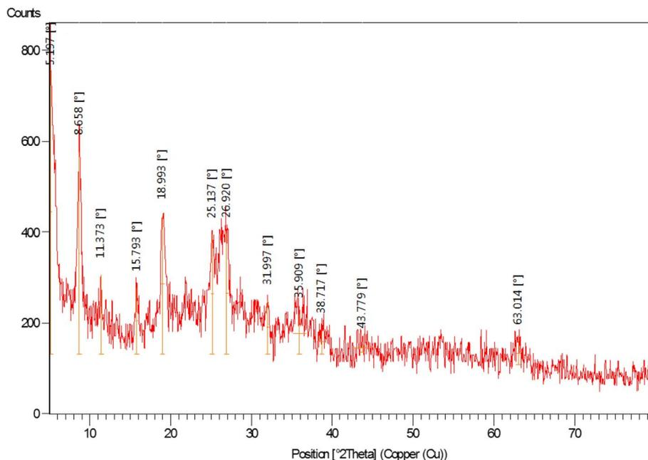
Fig. 5 The XRD spectrum of NGFRNH.
