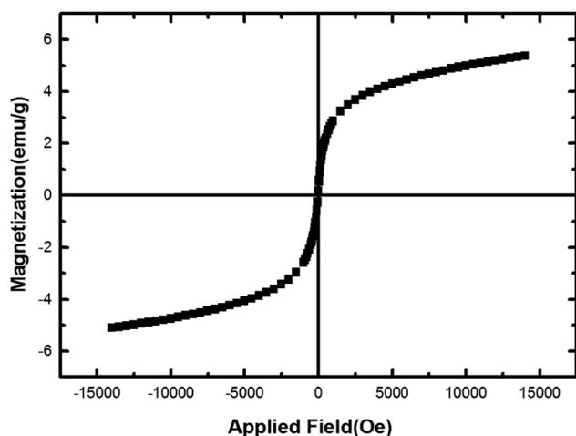
Fig. 7 The VSM diagram of the magnetic nanocomposite.
