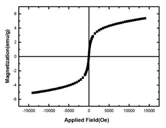
Fig. 7 The VSM diagram of the magnetic nanocomposite.
