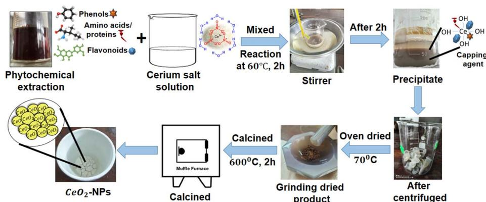
Fig. 2 Diagrammatic representation of the environmentally friendly synthesis of CeO<sub>2</sub>-NPs.
