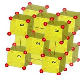
**Fig. 8** Shows the (a) Rietveld refinement graph; (b) electron density mapping in 2D counter form; (c) electron density mapping in 3D form; (d) crystal structure of CeO<sub>2</sub>-NPs in the single unit cell; (e) crystal structure of CeO<sub>2</sub>-NPs in a single layer; and (f) crystal structure in a polyhedral structure.
