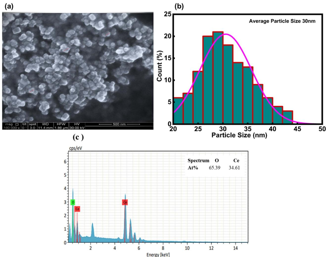
Fig. 6 (a) Shows the SEM of CeO<sub>2</sub>-NPs, (b) the average particle size distribution graph in nm, and (c) EDX analysis.
