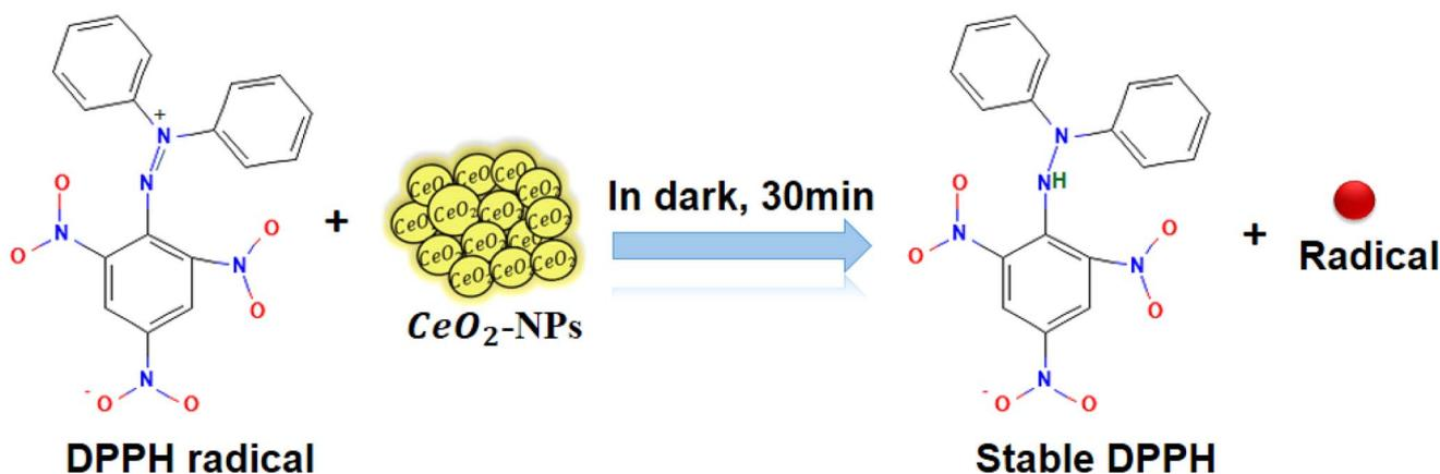
Fig. 11 Schematic mechanism of DPPH scavenging by CeO<sub>2</sub>-NPs.
