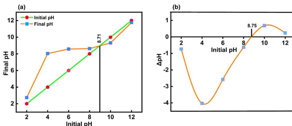
Fig. 10 (a and b) Shows typical plots used to determine the pH<sub>pzc</sub> of CeO<sub>2</sub>-NPs.
