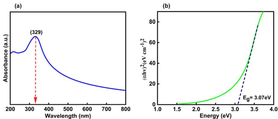
Fig. 4 Shows (a) UV-visible spectrum and (b) band gap of CeO<sub>2</sub>-NPs.
