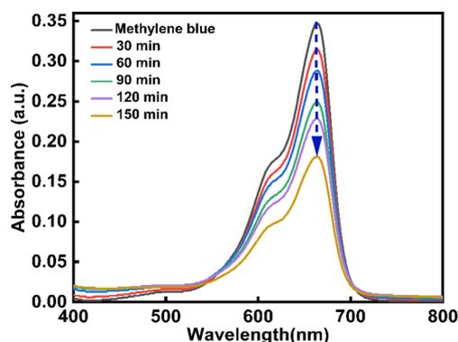
Fig. 16 Degradation of methylene blue dye by CeO<sub>2</sub>-NPs under UV irradiation.
