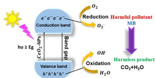
Fig. 17 Mechanism of photodegradation of MB dyes using CeO<sub>2</sub>-NPs.
