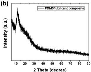
Fig. 3 Results of X-ray diffraction of (a) bare PDMS and (b) PDMS/ lubricant composite.
