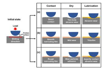
Fig. 11 Schematic illustration of the wear mechanisms on (a) non-coating, (b) lower xylene ratio (1:0) and (1:1), and (1:1), and (1:1) ratio (1:3), (1:1), and (1:1) PDMS/lubricant composite-coated aluminum surfaces under dry and lubricated conditions.
