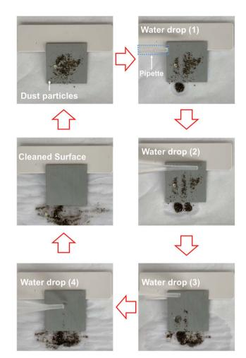
Fig. 12 Self-cleaning test of micro/nano-structured Al coated with PDMS/lubricant composite.
