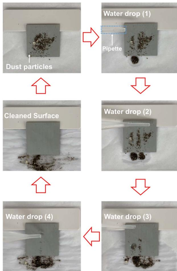
Fig. 12 Self-cleaning test of micro/nano-structured Al coated with PDMS/lubricant composite.
