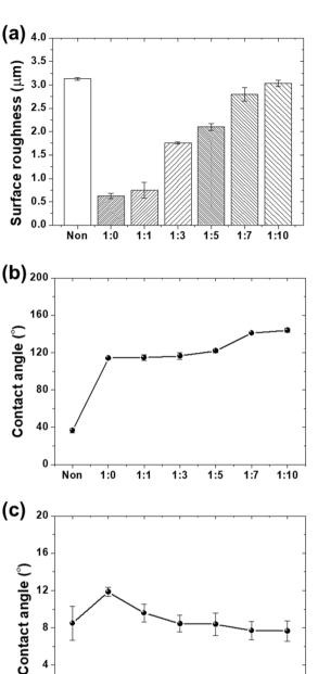
Fig. 5 Surface properties of micro/nano-structure surfaces coated with PDMS/lubricant composite at varying xylene dilution ratios: (a) surface roughness, (b) water contact angle and (c) oil contact angle.
