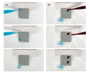
Fig. 13 Comparison of the wettability of water and oil droplets on micro/nano-structured Al coated with PDMS/lubricant composite: (a) water droplet, (b) oil droplet.
