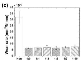
Fig. 7 Friction and wear characteristics of micro/nano-structure surfaces coated with PDMS/lubricant composite at varying xylene dilution ratios under dry condition: (a) friction coefficient history, (b) average friction coefficient and (c) wear rate.
