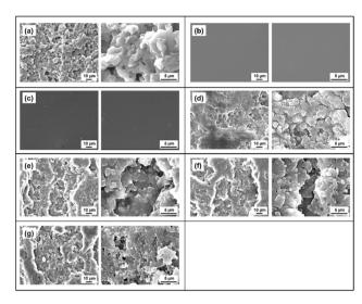
Fig. 2 SEM images of micro/nano-structured surfaces coated with PDMS/lubricant composites at varying xylene dilution ratios. Weight ratio of PDMS/lubricant composite: xylene is 1 to X, where X is (a) non-coating, (b) 0, (c) 1, (d) 3, (e) 5, (f) 7, (g) 10. (Left) Low magnification, (Right) high magnification.
