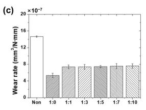
Fig. 9 Friction and wear characteristics of micro-nanostructure surfaces coated with PDMS/lubricant composite at varying xylene dilution ratios under lubrication condition: (a) friction coefficient history, (b) average friction coefficient and (c) wear rate.
