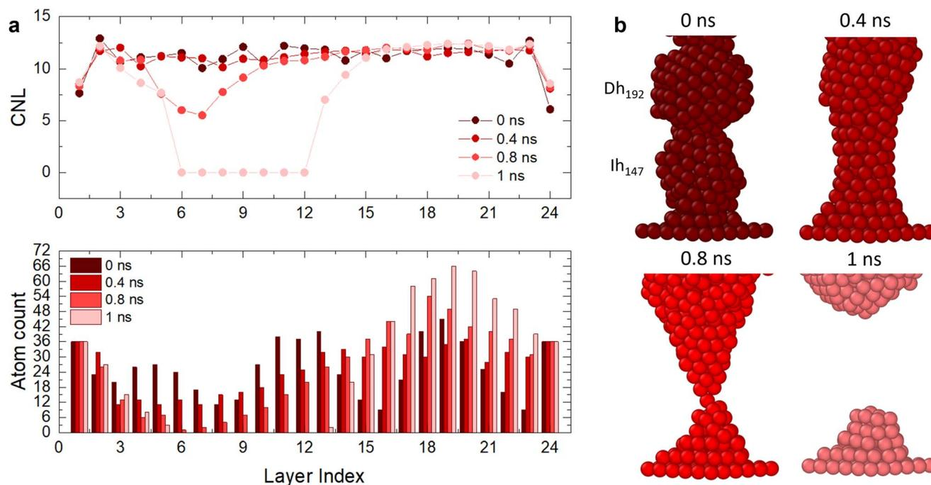
Fig. 5 (a) CNL and atom count per layer of (b) C.1, which has a Dh<sub>192</sub> in the middle, with length  $L_{\text{fixed},1} = 55 \text{ \AA}$ . The nanofilament breaks within 1 ns at the Ih/Dh interface. The Ih/Dh interface progressively diminishes from 12 to 0 atoms, indicating atom migration towards the electrodes. The break is characterized by a decrease in CNL from 11 (0 ns), to 10.5 (0.4 ns), to 6 (0.8 ns), to 0 at layer 6.
