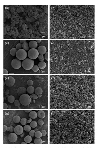
Fig. 3 SEM micrographs of the heat-treated zirconia samples. (a) and (b)  $\rm ZrO_2$  (monoclinic) after heat treated at 600 °C. (c) and (d) 3Y-TZP after heat treated at 1100 °C. (e) and (f) 4Y-TZP after heat treated at 1100 °C. (g) and (h) 6Y-TZP after heat treated at 1100 °C.
