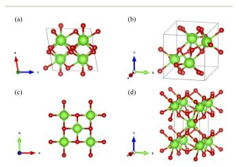
Fig. 1 Schematic illustrations of zirconia crystal structures.  $^{14}$  Green and red denote zirconia and oxygen atoms, respectively. (a) Monoclinic zirconia, view toward the b-axis. (b) Monoclinic zirconia, view toward the a-axis. (c) Tetragonal zirconia, view toward the c-axis. (d) Tetragonal zirconia, view toward the a-axis.
