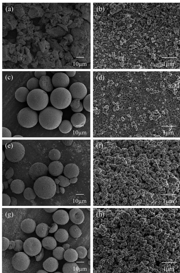
Fig. 3 SEM micrographs of the heat-treated zirconia samples. (a) and (b) ZrO<sub>2</sub> (monoclinic) after heat treated at 600 °C. (c) and (d) 3Y-TZP after heat treated at 1100 °C. (e) and (f) 4Y-TZP after heat treated at 1100 °C. (g) and (h) 6Y-TZP after heat treated at 1100 °C.
