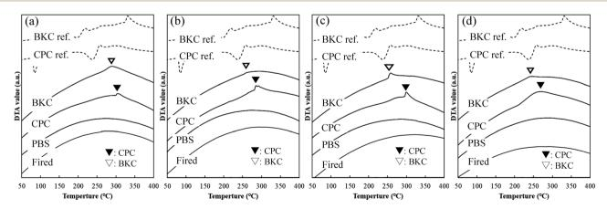
Fig. 5 DTA curves of each zirconia sample immersed in PBS, CPC, and BKC. (a)  $ZrO_2$ , (b) 3Y-TZP, (c) 4Y-TZP, and (d) 6Y-TZP. The CPC and BKC references are indicated by the dotted lines. The inverted triangular marks indicate the significant peaks of each sample immersed in CPC and BKC.
