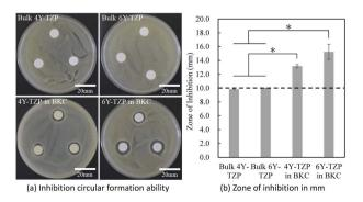
Fig. 7 Results of the antibacterial activity test of 4Y-TZP and 6Y-TZP absorbed with and without BKC against *S. aureus* (n=3). (a) Inhibition circular formation ability, (b) zone of inhibition in mm. The dotted line on (b) denotes the disc diameter. \*: p < 0.05.
