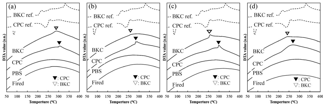
**Fig. 5** DTA curves of each zirconia sample immersed in PBS, CPC, and BKC. (a) ZrO<sub>2</sub>, (b) 3Y-TZP, (c) 4Y-TZP, and (d) 6Y-TZP. The CPC and BKC references are indicated by the dotted lines. The inverted triangular marks indicate the significant peaks of each sample immersed in CPC and BKC.
