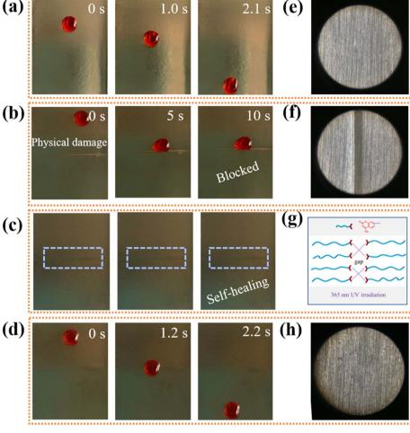
Fig. 4 Motion of a water droplet (20 μL) on the original SMEMG (a), SMEMG damaged *via* scalpel scratching, (b) and a self-healed SMEMG surface (d) under 365 nm UV light irradiation for 3 h; (c) a self-healed SMEMG surface under 365 nm UV light irradiation for 3 h. Optical microscopy images of original SMEMG (e), damaged SMEMG (f) and self-healed SMEMG surface (h). (g) Self-healing mechanism of damaged SMEMG under 365 nm UV light irradiation. The water droplet was dyed with methyl orange.
