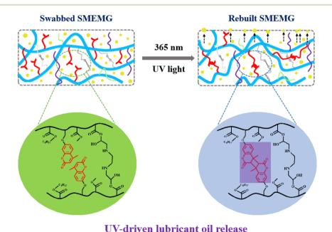
Fig. 9 Lubricant oil self-replenishing mechanism of the SMEMG.
