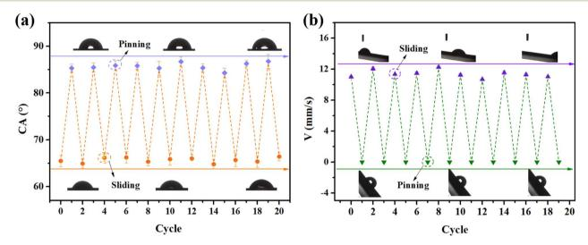
Fig. 10 CA (a) and sliding velocity (b) changes on the SMEMG as a function of repeated swabbing and UV light irradiation at 365 nm wavelength for 3 h; inset images in (a) show the CA images and in (b) the water droplet sliding motion on the SMEMG.
