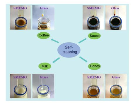
Fig. 5 Snapshots showing the sliding motion of coffee, sauce, milk, and honey droplets (~20 μL) on the SMEMG and glass.
