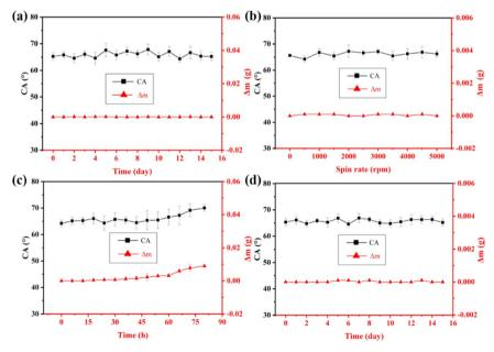
Fig. 6 Durability of the SMEMG. Variation of the CA and  $\Delta$ m of the SMEMG during the stability test. (a) SMEMG after heating at 80 °C for 1–15 days; (b) SMEMG rotated at 0–5000 rpm for 1 min; (c) SMEMG after immersing in water with a spin rate of 30 rpm for 80 h; (d) SMEMG placed in the vertical position for 1–15 days.
