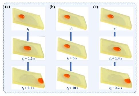
Fig. 7 Dynamic control of the mobility of a water droplet (20 μL) on the SMEMG. (a) Process of a water droplet slipping off the SMEMG at the initial state. (b) Process of a water droplet pinned on the SMEMG after the surface lubricant oil was swabbed. (c) Process of a water droplet resliding down the SMEMG after UV irradiation for 3 h.
