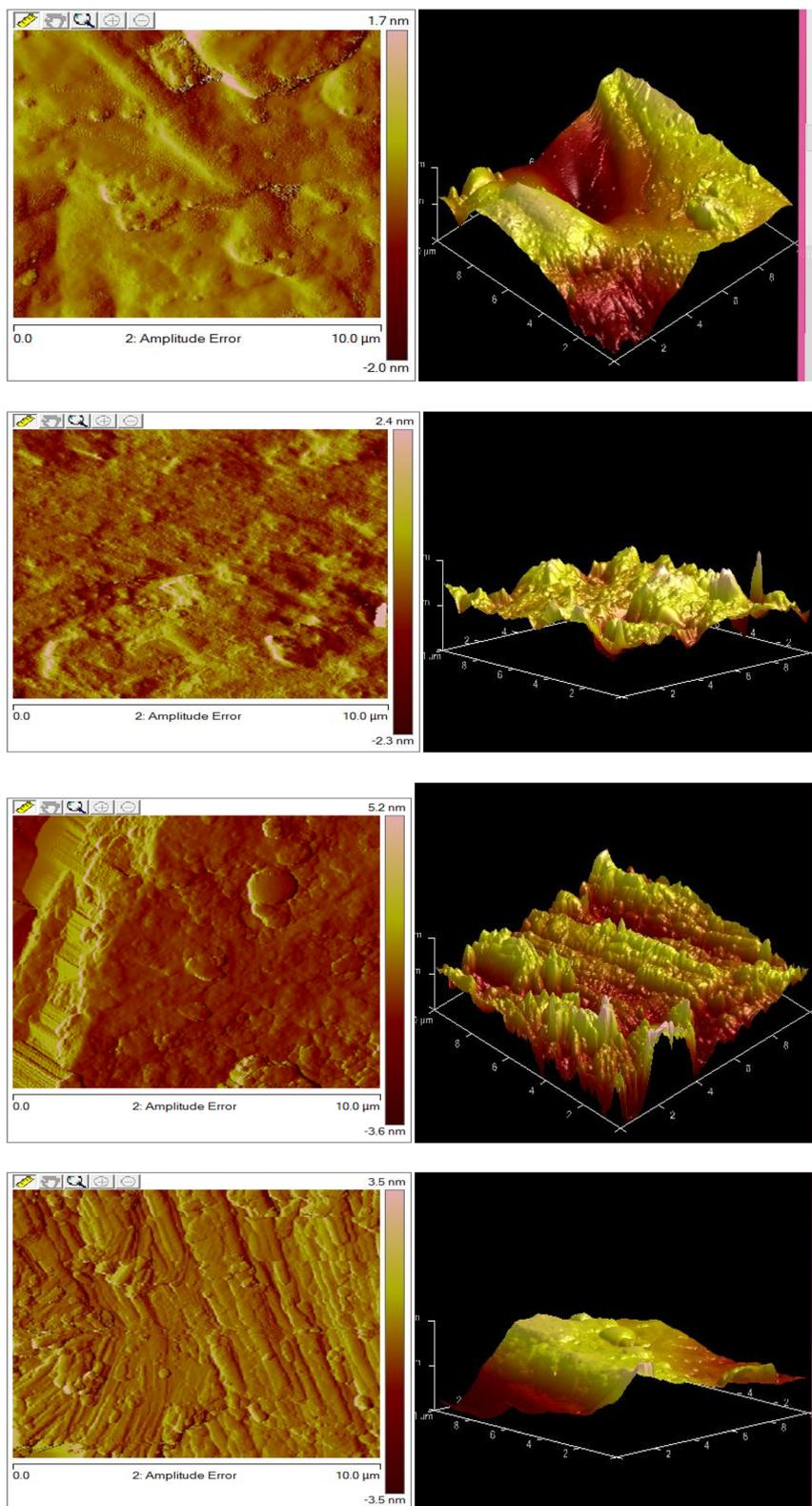
**Fig. 10** (a): AFM Corroded surface of casted Mg-0.5 wt% CNTs/0 wt% h-BN nanohybrid composites. (b): AFM Corroded surface of casted Mg-0.5 wt% CNTs/2 wt% h-BN nanohybrid composites. (c): AFM Corroded surface of casted Mg-0.5 wt% CNTs/4 wt% h-BN nanohybrid composites. (d): AFM Corroded surface of casted Mg-0.5 wt% CNTs/6 wt% h-BN nanohybrid composites.
