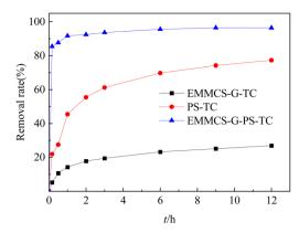
Fig. 3 The comparison of TC removal in different systems (TC concentration: 50 mg L<sup>-1</sup>; T = 25 °C; pH = 3; EMMCS-G: 15 mg).
