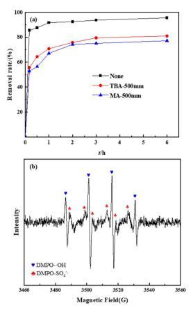
Fig. 7 (a) Effect of radical scarvengers on the TC removal. (b) EPR pattern of  $SO_4^{-1}$  and  ${}^{\bullet}OH$ .
