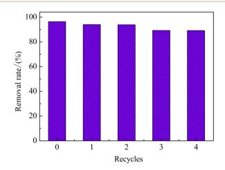
Fig. 6 TC and TOC removal in different recycles. (TC concentration: 50 mg  $\rm L^{-1}$ ; T=25 °C; PS concentration, 20 mM; pH = 3).
