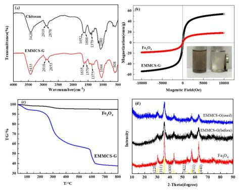
Fig. 2 (a) FTIR spectra of chitosan and EMMCS-G. (b) Magnetic hysteresis loops of  $Fe_3O_4$  and EMMCS-G. (c) TGA curves of  $Fe_3O_4$  and EMMCS-G. (d) XRD patterns of  $Fe_3O_4$  and EMMCS-G before and after reaction in EMMCS-G/PS system.
