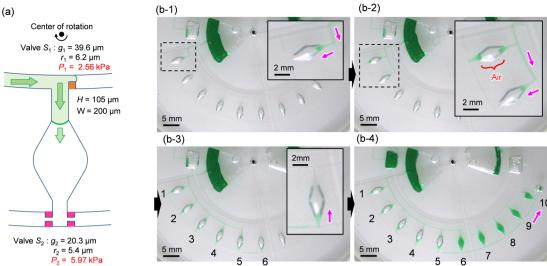
Fig. 2 Schematic representation of a method for outward sequential liquid dispensing into an array of 10 microchambers along the direction of centrifugal force. (a) Detailed design of the microchamber integrated with a pair of passive stop valves with different burst pressures. (b) Experimental results showing liquid dispensing into the microchambers at a rotational speed of 1500 min<sup>-1</sup>.
