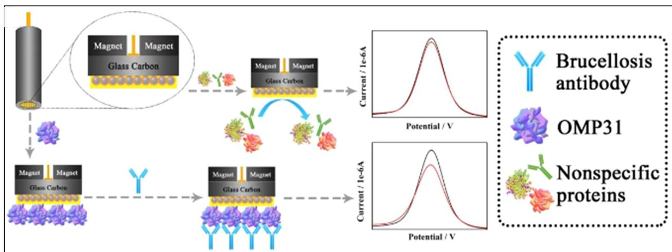
Fig. 12 Schematic diagram explaining the fabrication of Fe<sub>3</sub>O<sub>4</sub>@Au@PEG@HA NPs electrochemical immunosensor. The figure was adapted from ref. 190 and reproduced with permission, copyright @ Elsevier.
