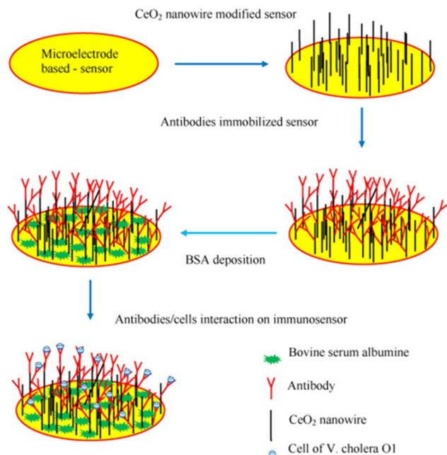
Fig. 6 Schematic illustration of the immunosensor fabrication for the detection of *V. cholera* O1 detection. The figure was adapted from ref. 133 and reproduced with permission, copyright @ Elsevier.
