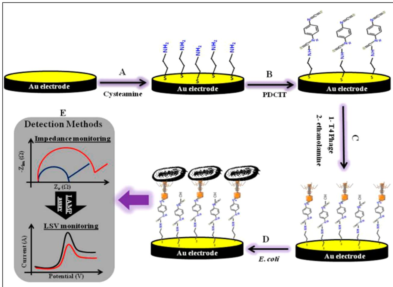
Fig. 5 Schematic illustration showing the fabrication of AuE/Cys/PDCIT/T<sub>4</sub> phage electrode. The figure was adapted from ref. 122 reproduced with permission, copyright @ Elsevier.
