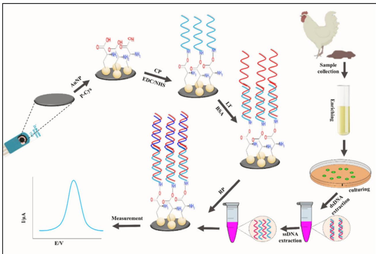
Fig. 4 Schematic illustration for the fabrication of DNA-biosensor and the detection of *Salmonella Typhi* from real samples. The figure was adapted from ref. 102 and reproduced with permission, copyright @ Elsevier.
