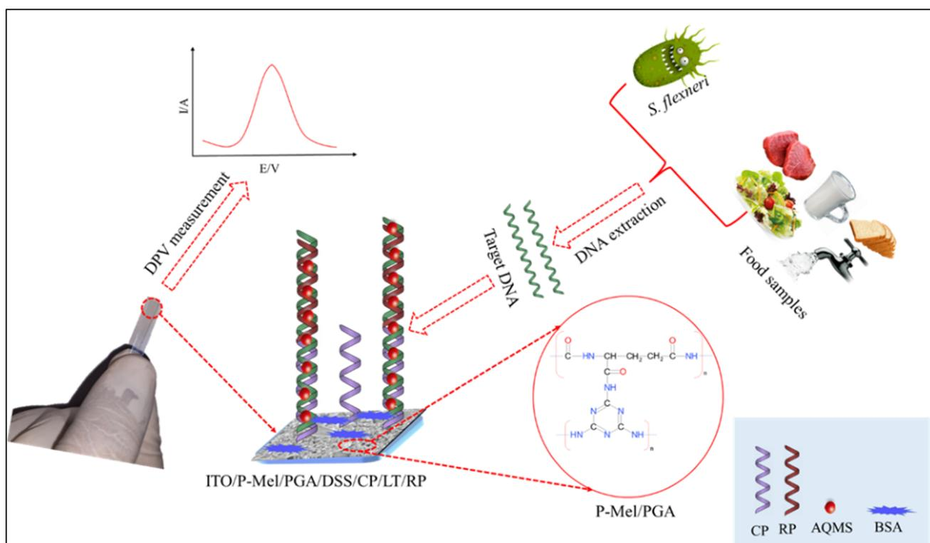
Fig. 7 Schematic diagram illustrating the fabrication process of the ITO/P-Mel/PGA/DSS modified electrode for the detection *Shigella flexneri*. The figure was adapted from ref. 137 and reproduced with permission, copyright @ Elsevier.
