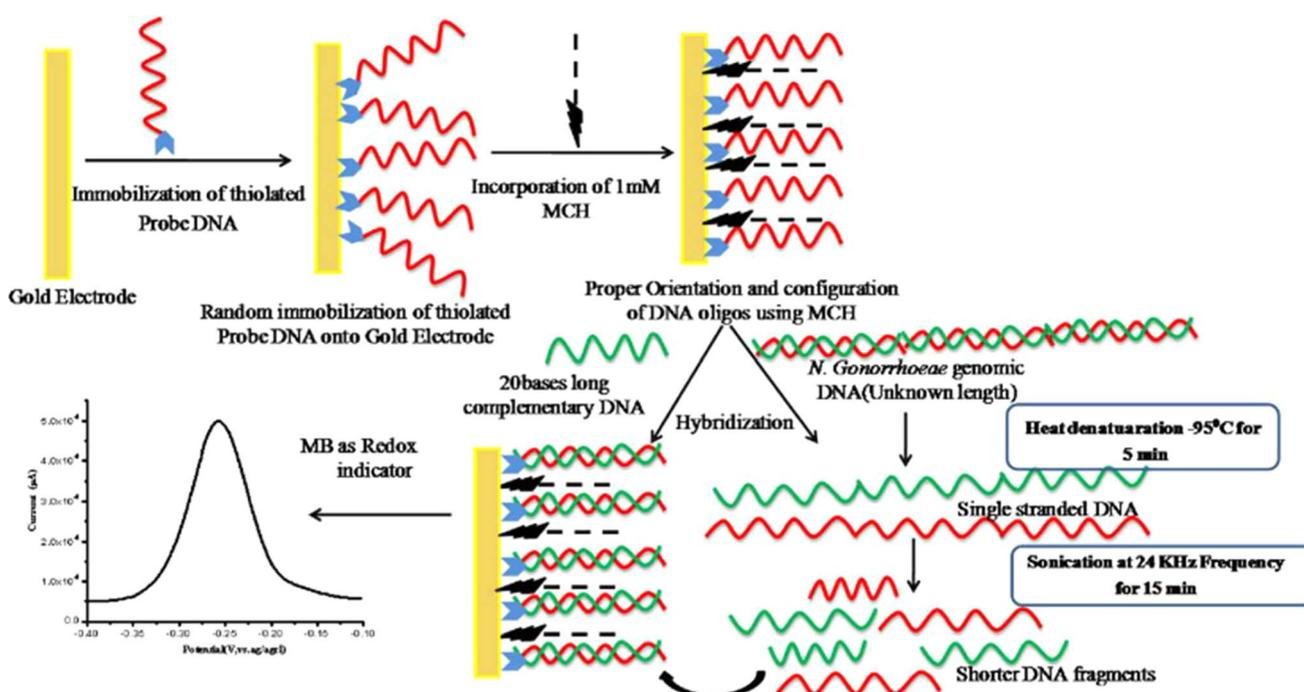
Fig. 8 Schematic diagram showing the fabrication process of the ssDNA-Au electrode for the detection of *Neisseria gonorrhoeae*. The figure was adapted from ref. 150 and reproduced with permission, copyright @ Elsevier.
