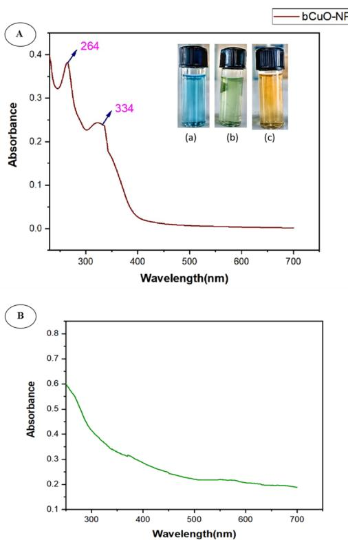
Fig. 1 (A) UV-vis spectrum of bCuO-NPs, (B) UV-vis spectrum of plant extract.
