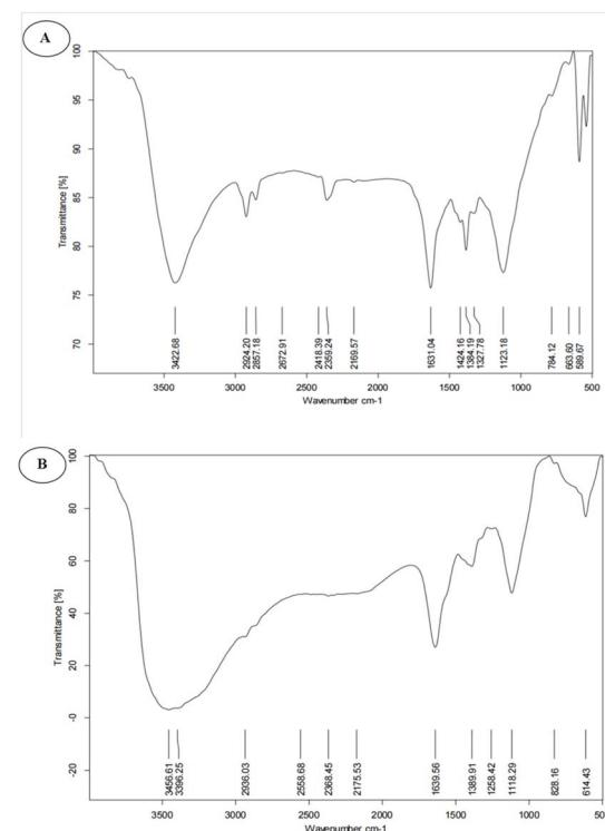
Fig. 2 (A) FT-IR spectrum of bCuO-NPs, and (B) zaluzaanin-D enriched *Vernonia arborea* ethyl acetate extract.
