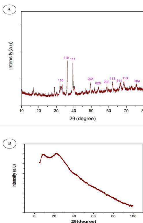
Fig. 3 (A) XRD pattern of bCuO-NPs showed intense peaks at specific 2 theta values and (B) plant extract.
