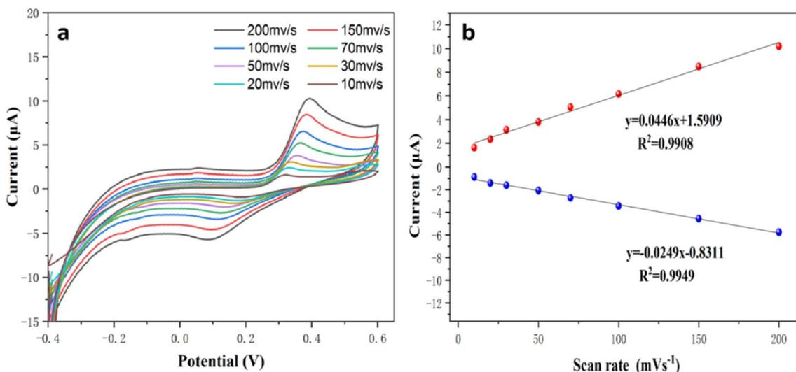
Fig. 10 (a) The different scan rate CV performances using PA-CoMn-1 : 1.5 : 0.5 aerogel/SPCE from the range of 10 to 200 mV s<sup>-1</sup> and (b) their scan rate against its current response linear plot.
