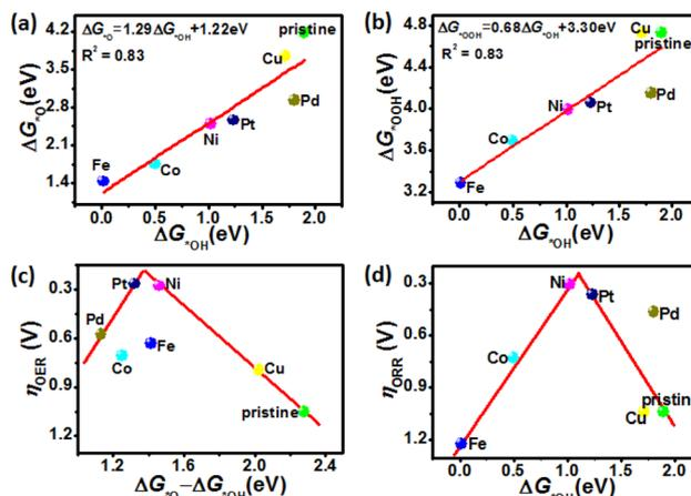
Fig. 6 Scaling relationship between the adsorption-free energies of (a)  $\Delta G_{*OH}$  vs.  $\Delta G_{*O}$  and (b)  $\Delta G_{*OH}$  vs.  $\Delta G_{*OOH}$  on the surface of pristine and TM-doped ZnS nanostructures. The volcano plot of (c)  $\eta^{OER}$  vs.  $\Delta G_{*O} - \Delta G_{*OH}$  and (d)  $\eta^{ORR}$  vs.  $\Delta G_{*OH}$  for OER and ORR on the surface of pristine and TM-doped ZnS nanostructures.
