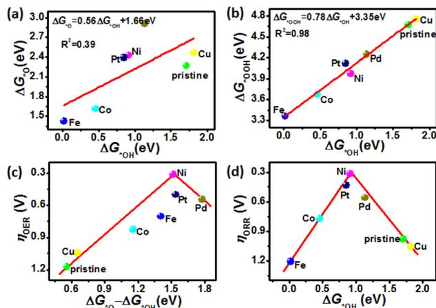
Fig. 7 Scaling relationship between the adsorption-free energies of (a)  $\Delta G_{*OH}$  vs.  $\Delta G_{*O}$  and (b)  $\Delta G_{*OH}$  vs.  $\Delta G_{*OOH}$  on the surface of pristine and TM-doped ZnSe nanostructures. The volcano plot of (c)  $\eta_{OER}$  vs.  $\Delta G_{*O} - \Delta G_{*OH}$  and (d)  $\eta_{ORR}$  vs.  $\Delta G_{*OH}$  for OER and ORR on the surface of pristine and TM-doped ZnSe nanostructures.
