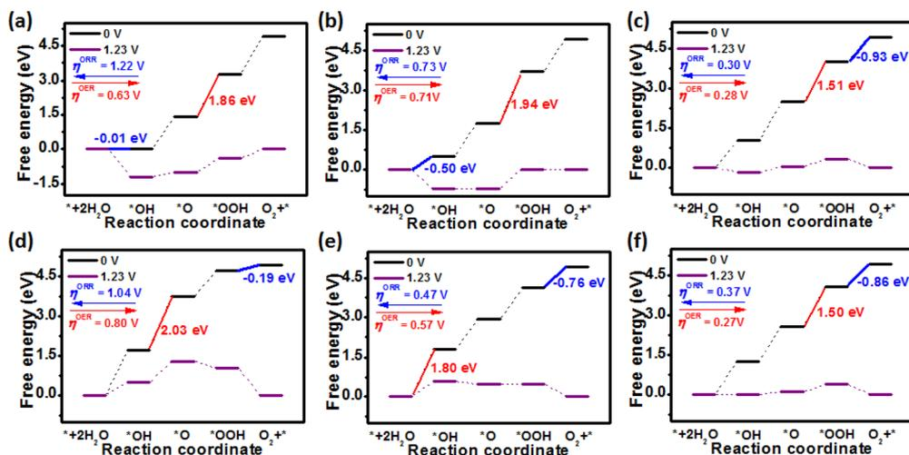
Fig. 4 Free energy diagram of (a) Fe, (b) Co, (c) Ni, (d) Cu, (e) Pd and (f) Pt-doped ZnS nanostructures for OER and ORR at  $U = 0$  and 1.23 V, respectively. The red and blue lines are the potential-determining steps (PDS) for OER and ORR.
