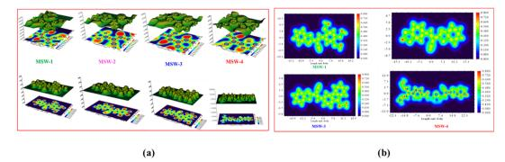
Fig. 5 (a) ELF maps of the co-sensitizer benzoxalylacetonitrile sensitizer MSW-1-4, (b) localized orbital locator maps (LOL) for the optimized geometry of the co-sensitizer oxazolylacetonitrile MSW-1-4.
