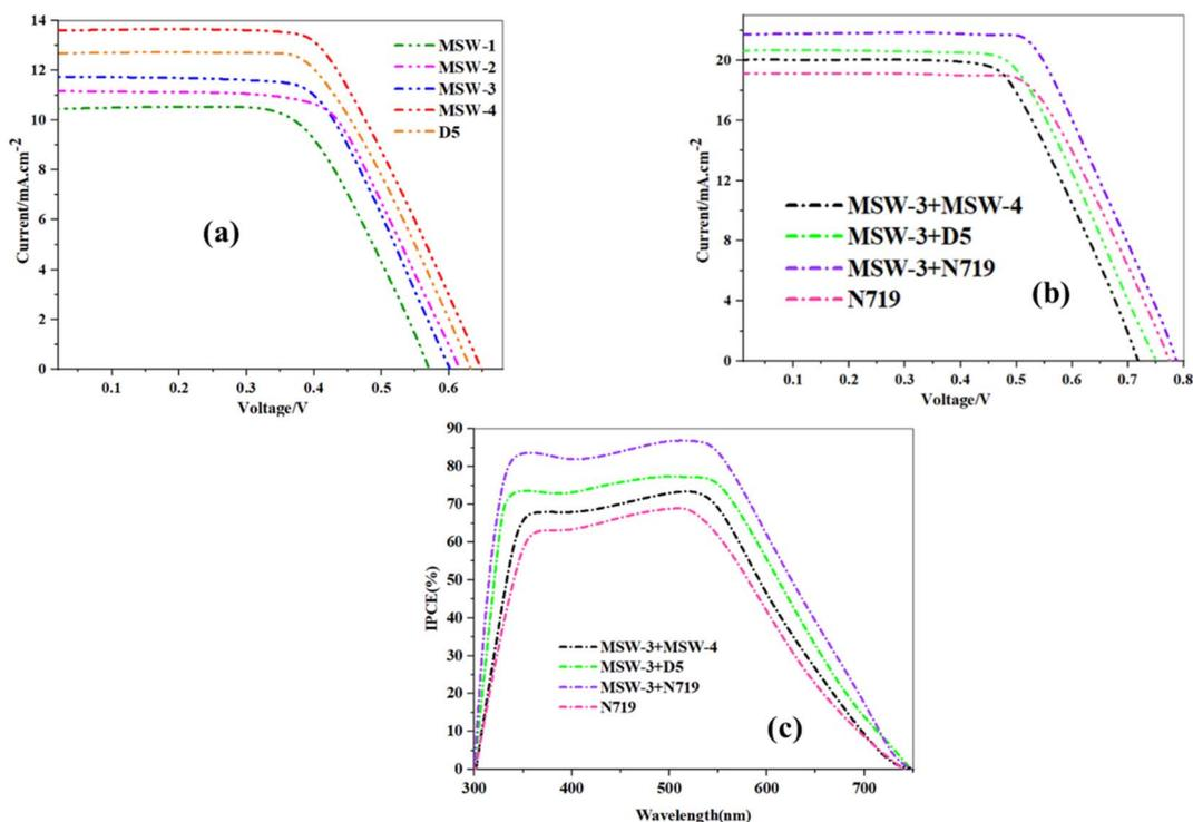
Fig. 7 (a)  $J$ - $V$  curves of benzoxalacetonitrile sensitizer **MSW-1-4** devices, (b)  $J$ - $V$  curves of **MSW-3-4**, **D-5**, and **N719**, (c) IPCE spectra of **MSW-3-4**, **D-5**, **MSW-4** and **N719**.
