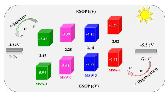
Fig. 6 Energy level diagram of the benzoxalylacetonitrile sensitizer MSW-1-4.
