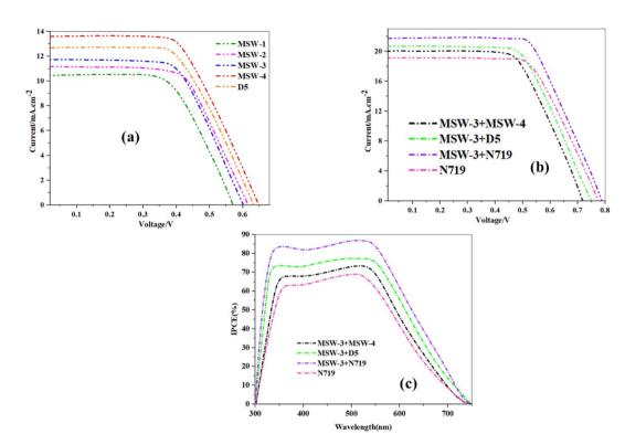
Fig. 7 (a) J-V curves of benzoxalylacetonitrile sensitizer MSW-1-4 devices, (b) J-V curves of MSW-3-4, D-5, and N719, (c) IPCE spectra of MSW-3-4, D-5, MSW-4 and N719.
