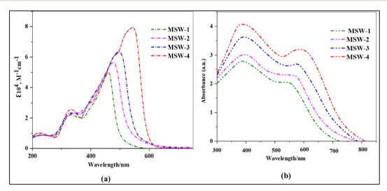
Fig. 2 (a) UV-Vis absorption of benzoxalylacetonitrile (BOA) sensitizer MSW-1-4 in solution, (b) Absorption of the sensitizer MSW-1-4 on TiO<sub>2</sub>.
