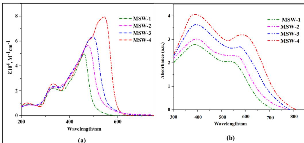
Fig. 2 (a) UV-Vis absorption of benzoxalacetonitrile (BOA) sensitizer MSW-1-4 in solution, (b) Absorption of the sensitizer MSW-1-4 on TiO<sub>2</sub>.
