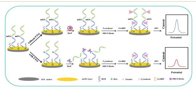
Scheme 1 Electrochemical detection schematic for FTO based on the specific cleavage action of MazF and signal amplification of HRP.
