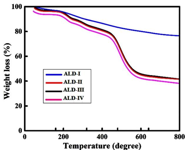
Fig. 4 TGA illustration of newly developed films.
