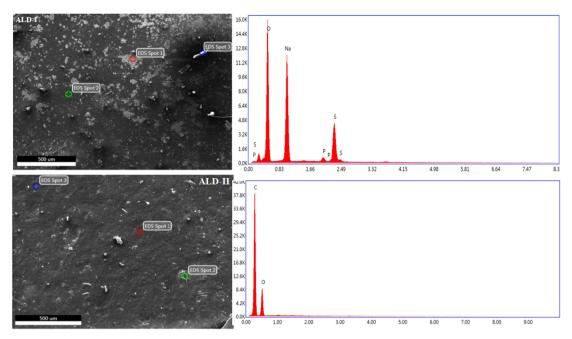
Fig. 10 EDS illustration of newly developed biodegradable films (ALD-I and ALD-II).
