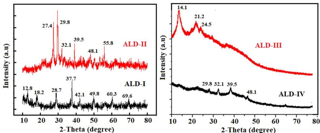
Fig. 3 XRD pattern of newly developed biodegradable films.
