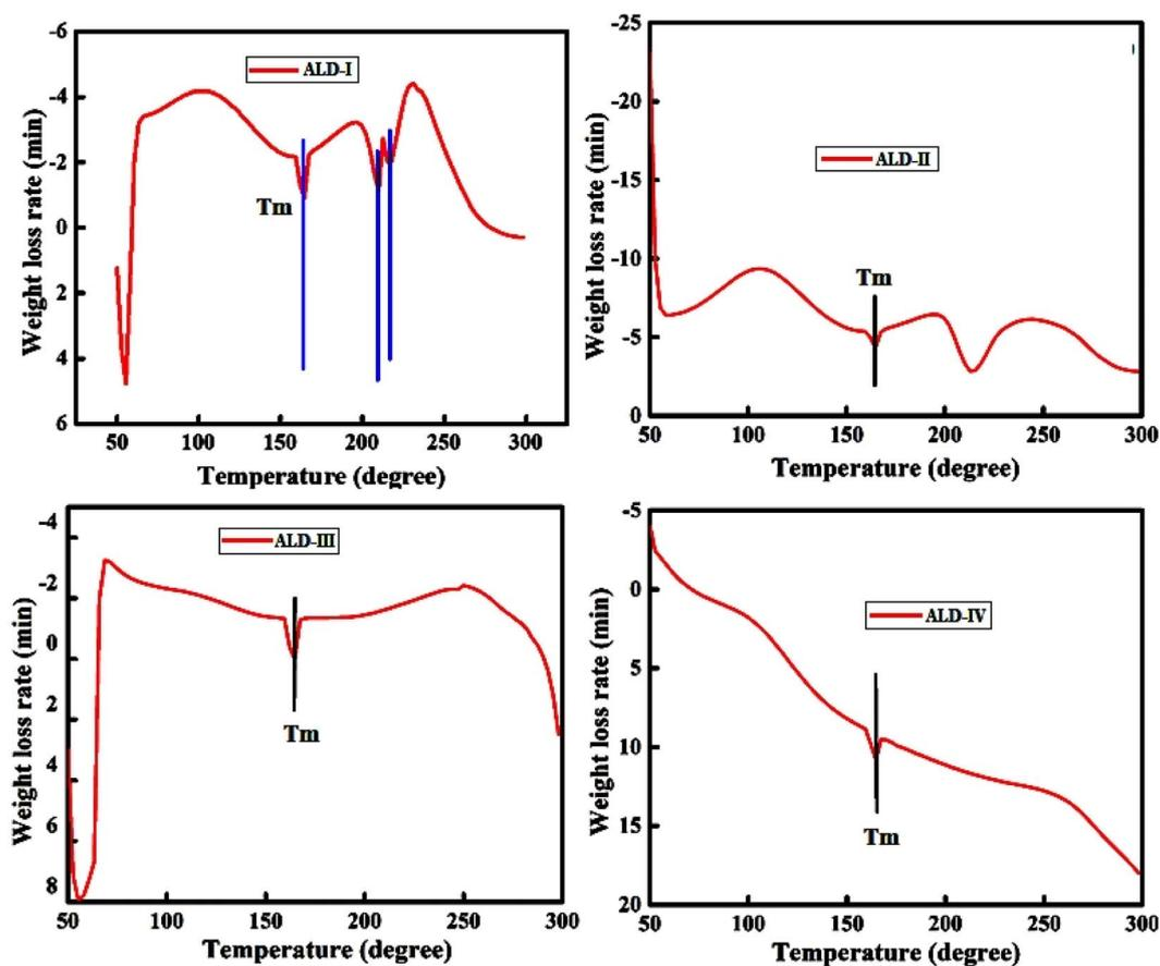
Fig. 5 DSC illustration of newly developed films.
