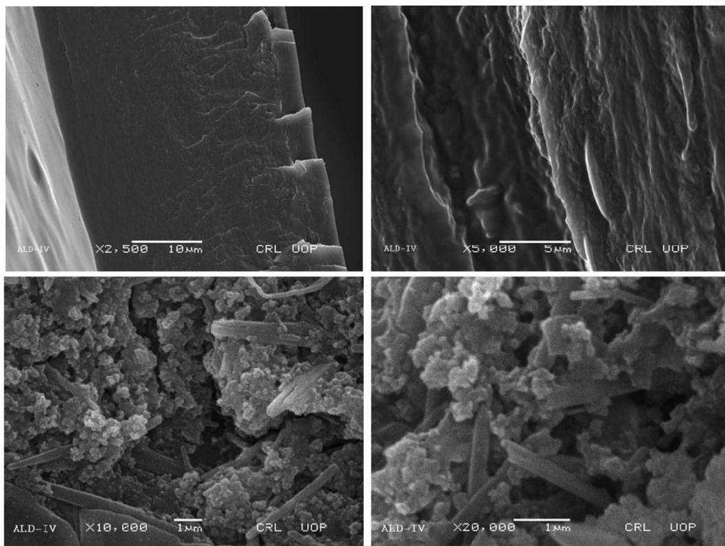
Fig. 9 Surface morphology of newly developed film (ALD-IV) illustrated by SEM.
