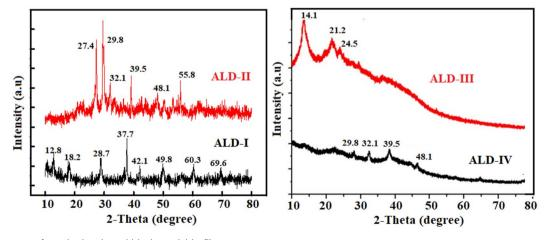
Fig. 3 XRD pattern of newly developed biodegradable films.
