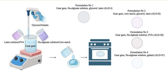
Fig. 1 Schematic layout for the preparation of biodegradable films.
