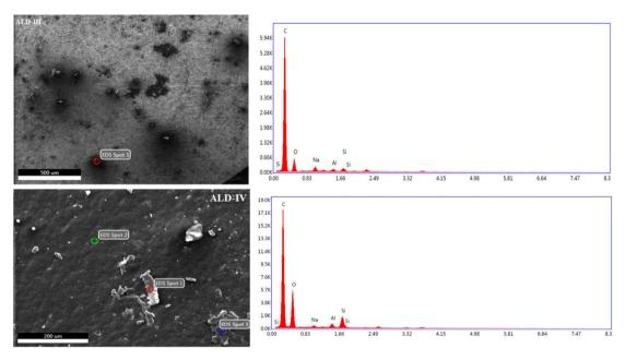
Fig. 11 EDS illustration of newly developed biodegradable films (ALD-III and ALD-IV).
