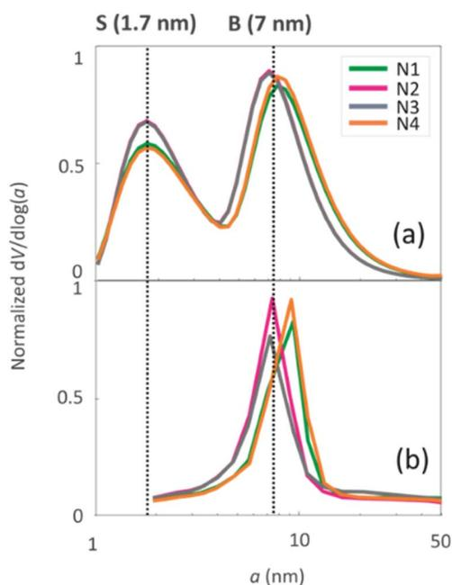
Fig. 5 Pore size distributions of the four geopolymers derived from (a) <sup>1</sup>H cryoporometry NMR data and (b) N<sub>2</sub> desorption data analysed with the BJH method.
