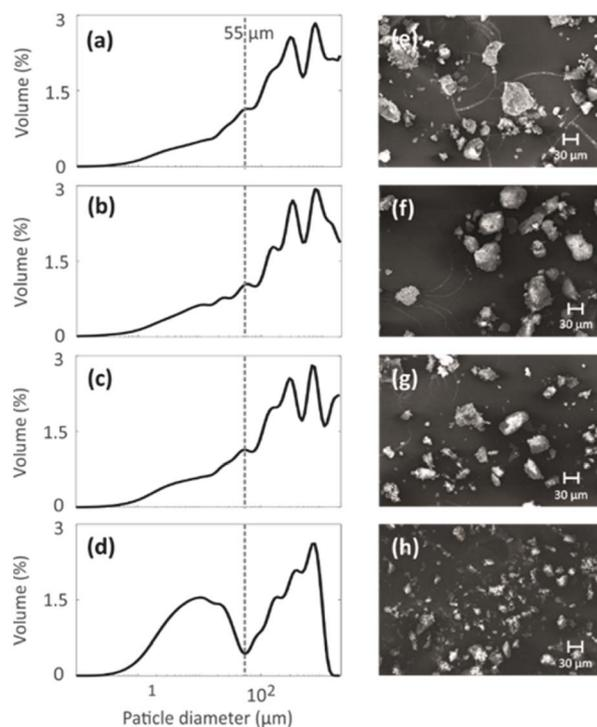
**Fig. 4** (a–d) Particle size distributions and (e–h) SEM images of four geopolymers with different NH<sub>4</sub>OH post-treatment times: (a and e) 0 min (N1), (b and f) 15 min (N2), (c and g) 3 h (N3) and (d and h) 24 h (N4).
