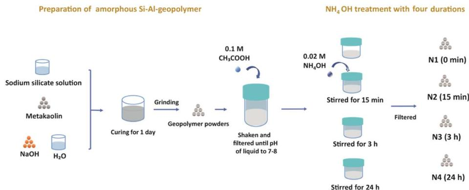
Fig. 1 The procedure for sample preparation.
