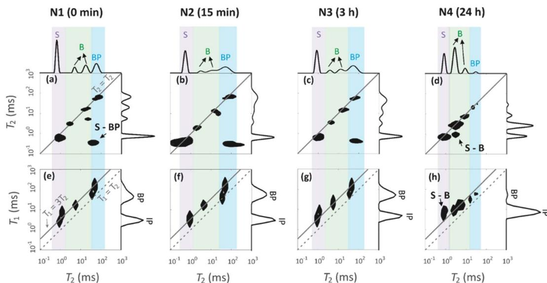
Fig. 7 (a–d)  $^1\text{H}$   $T_2$ - $T_2$  exchange spectra of water in the geopolymer samples measured with mixing time of 0.2 ms. (e–h)  $^1\text{H}$   $T_1$ - $T_2$  correlation spectra.  $T_2$  and  $T_1$  distributions measured using CPMG and saturation recovery experiments are shown on the top and right of the 2D plots.
