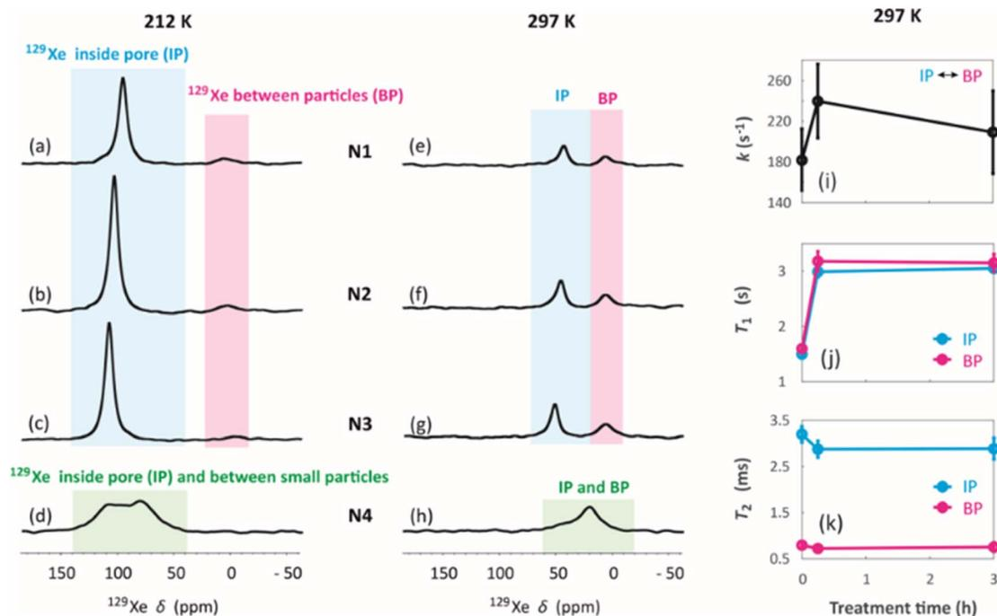
Fig. 6  $^{129}\text{Xe}$  NMR spectra of (a and e) N1, (b and f) N2, (c and g) N3 and (d and h) N4 measured at (a–d) 212 K and (e–h) 297 K. (i) Exchange rates of Xe between the intra particle and inter particle sites in samples N1, N2 and N3 determined using selective inversion recovery experiments. (j)  $T_1$  and (k)  $T_2$  relaxation times of  $^{129}\text{Xe}$  in N1, N2 and N3 samples.
