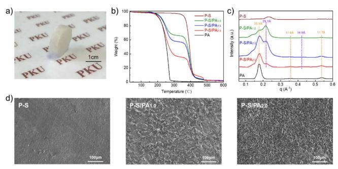
Fig. 1 (a) Photograph of P-S/PA; (b) TG curves, (c) one-dimensional curves of WAXS and (d) SEM images of P-S/PA with different PA contents.
