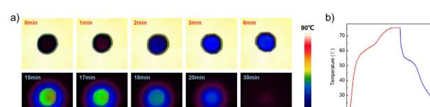
(a) Real-time IR images of P-S/PA; (b) temperature-time curves of P-S/PA
