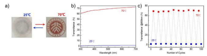
Fig. 4 (a) Photographs of P-S/PA at 25 °C and 70 °C; (b) transmittance of P-S/PA at 25 °C and 70 °C; (c) transmittance (@600 nm) of P-S/PA after multiple cycles.
