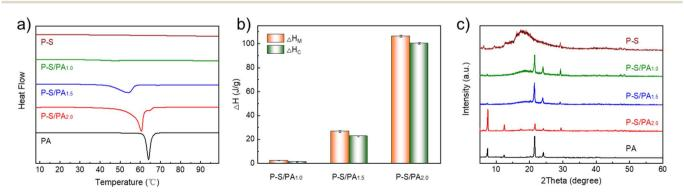
Fig. 2 (a) DSC heating curves of P-S/PA with different PA contents; (b) melting enthalpy  $\Delta H_{\text{M}}$  and crystallization enthalpy  $\Delta H_{\text{C}}$  of P-S/PA; (c) XRD diagrams of P-S/PA.
