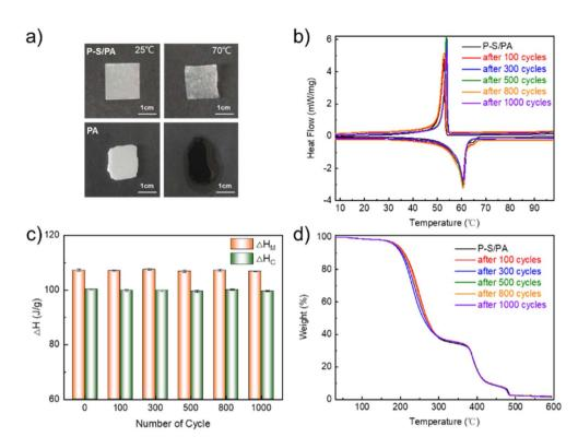
Fig. 3 (a) Photographs of P–S/PA and PA at 25 °C and 70 °C; (b) DSC curves (c) melting enthalpy  $\Delta H_{M}$  and crystallization enthalpy  $\Delta H_{C}$  and (d) TG curves of P–S/PA after multiple thermal cycles.
