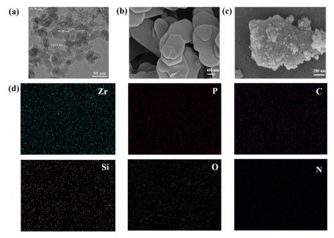
Fig. 2 TEM image of SiO<sub>2</sub> (a), SEM images of  $\alpha$ -ZrP (b), PDA@ $\alpha$ -ZrP/SiO<sub>2</sub> (c) and EDS mapping of PDA@ $\alpha$ -ZrP/SiO<sub>2</sub> (d).
