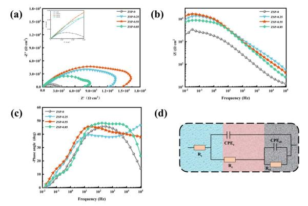
EIS Nyquist plots (a), EIS Bode plots of different phosphate coatings (b and c), and the equivalent electrical circuit (d).
