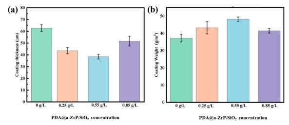
Phosphate coatings thickness (a) and weight (b) with different PDA@α-ZrP/SiO<sub>2</sub> concentration.
