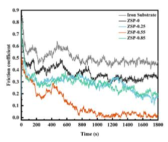
Fig. 6 Friction coefficients curves of phosphate coatings under 100 rpm and a fixed load of 100 N for 30 min at ambient temperature.
