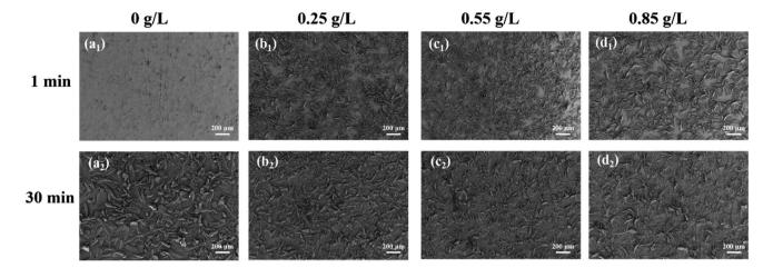
Fig. 3 SEM images of phosphate coatings with different PDA@α-ZrP/SiO<sub>2</sub> concentration as a function of time.
