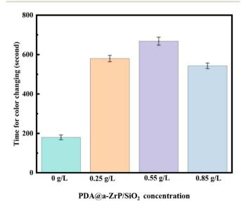
Fig. 9 The time for color changing of samples in copper sulfate dropping experiments.
