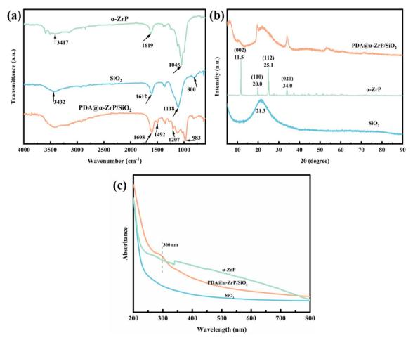
Fig. 1 FT-IR spectra (a), XRD spectra (b) and UV-vis spectra (c) for SiO<sub>2</sub>, α-ZrP and PDA@α-ZrP/SiO<sub>2</sub>
