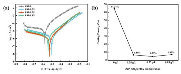
Fig. 7 Potentiodynamic polarization curves (a) and coating porosity (b) of phosphate coatings with different content of PDA@α-ZrP/SiO<sub>2</sub>.
