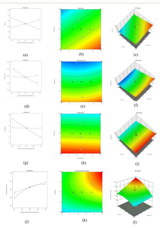
Fig. 4 Perturbation plot (a, d, g, and j), contour plot (b, e, h, and k), and 3-D response plot (c, f, I, and I) for peak area, retention time, tailing factor and theoretical plate number of irbesartan respectively.
