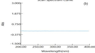
Fig. 8 (a) HPLC chromatogram of distilled ethanol. (b) UV spectrum of the distilled ethanol using HPLC grade ethanol as a blank.
