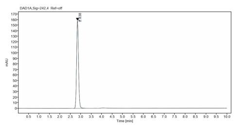
Fig. 2 Standard chromatogram of irbesartan (50  $\mu$ g mL<sup>-1</sup>) at Rt 2.83 min.
