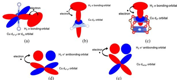
Fig. 9 Possible schemes of forward electron donation from a  $H_2$   $\sigma$  boding orbital to open copper sites in the L(CuL<sub>2</sub>) (a), T(CuL<sub>3</sub>) (b) and P(CuL<sub>4</sub>)<sub>2</sub> (c) coordinations and electron back donation from Cu  $d_{x^2-y^2}$  (d) and  $d_{xz/yz}$  (e) orbitals to a  $H_2$   $\sigma^*$  anti-boding orbital. Red and blue lobes represent positive and negative values of wavefunctions, respectively.
