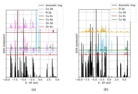
Fig. 4 (a) PDOS of the  $T(CuL_3)$  cluster with the top, middle and bottom layers representing the PDOS of the aromatic ring,  $CuN_3$  triangle in the  $T(CuL_3)$  coordination and  $ZnN_4$ , tetrahedron, respectively. (b) PDOS of the  $P(CuL_4)_2$  cluster with the top, middle and bottom layers representing the PDOS of the aromatic ring, Cu atom and C 2p states, respectively.
