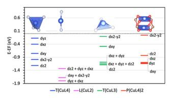
Fig. 7 Reduced diagrams quantitatively illustrating the ligand field splitting of Cu 3d states in the tetragonal coordination  $T(CuL_4)$ , linear coordination  $L(CuL_2)$ , triangle coordination  $T(CuL_3)$  and paddlewheel coordination  $P(CuL_4)_2$  from left to right, respectively.
