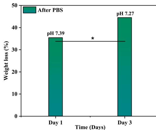
Fig. 15 Statistical analysis (ANOVA  $p < 0.05$ ) of degradability of composite coatings in PBS at 7.41 pH. The difference between the degradability of coatings is significant (\*) between day 1 and day 3.
