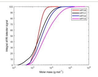
Fig. 1 Cumulative molar mass distribution of the synthesized hyperbranched polymers based on SEC-MALLS.
