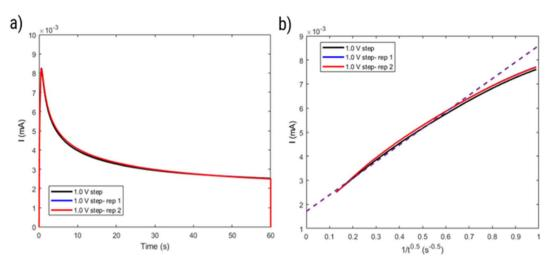
Fig. 9 (a) Current as a function of time and (b) current as a function of inverse square root of time obtained from a step potential chronoamperometry test on HPT-II1Cl (5.7 mM active TEMPO) in 1.5 M NaCl solution at pH = 2.0.
