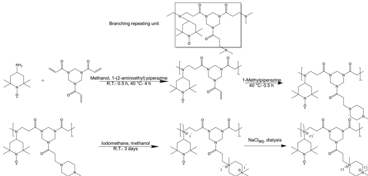
**Scheme 1** Schematic representation of the polymerization of 4-amino TEMPO and 1,3,5-triacryloylhexahydro-1,3,5-triazine and termination (first row). Post-polymerization modification of polymers through amine quaternization and ion exchange (second row).
