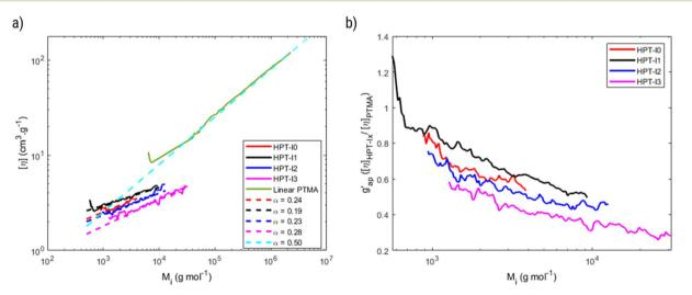
Fig. 2 (a) Double logarithmic plot of the intrinsic viscosity [ $\eta$ ] against the molar mass,  $M_i$ , for the hyperbranched polymers and a linear TEMPO-based polymer analogue (PTMA) based on SEC with viscometric detection. (b) Apparent contraction factor, defined as the ratio of the intrinsic viscosity of the hyperbranched polymers to that of PTMA, as a function of molar mass.
