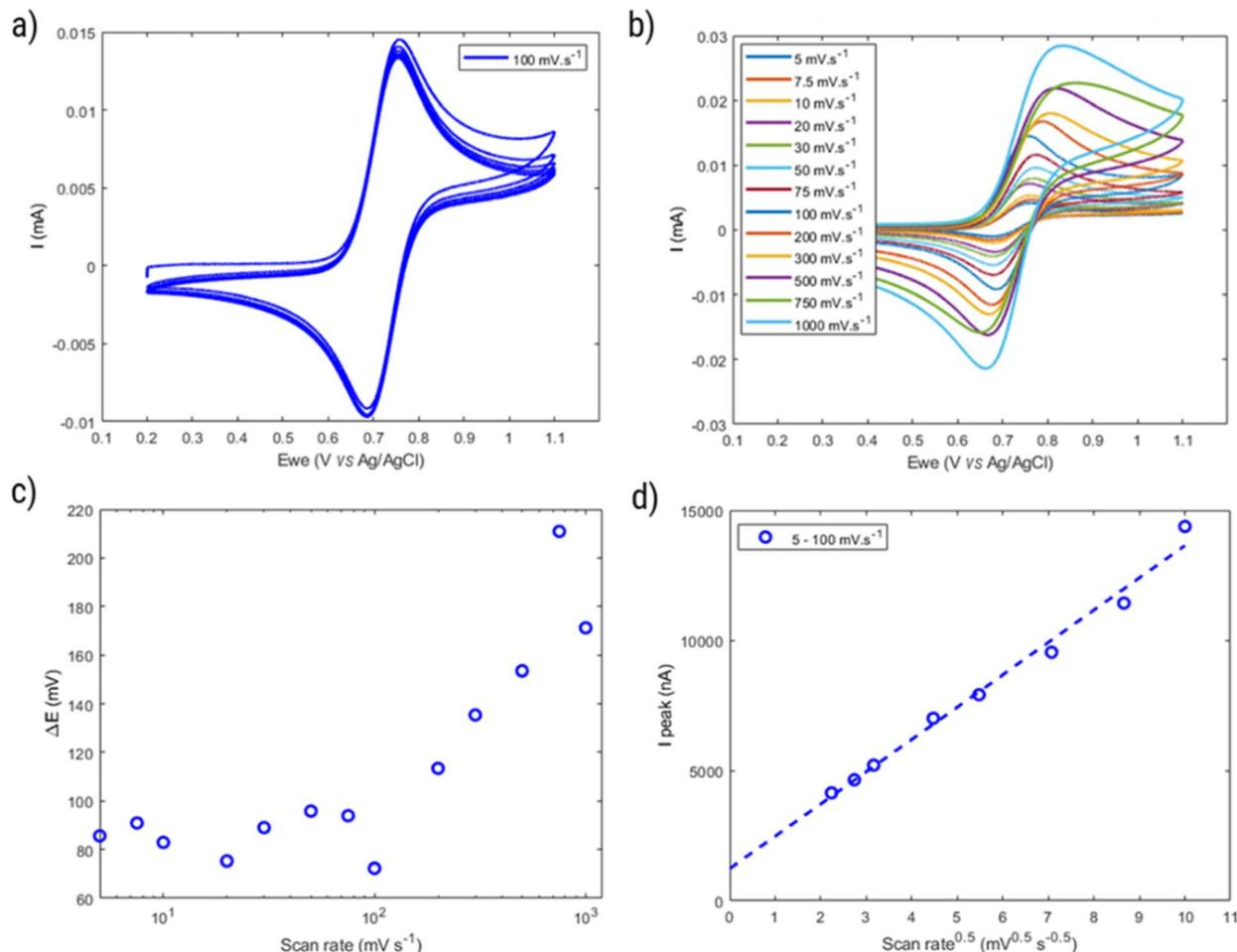
**Fig. 8** (a) Cyclic voltammogram of HPT-II1Cl (5.7 mM active TEMPO) in 1.5 M NaCl aqueous solution at pH = 2.0 and at the scan rate of 100 mV s<sup>-1</sup> (six consecutive cycles). (b) First cycle voltammograms at various scan rates. (c) Peak-to-peak potential difference (obtained from the first cycle voltammograms) as a function of scan rate. (d) Oxidation peak current as a function of square root of scan rate in the reversible range (scan rates of 5 to 100 mV. s<sup>-1</sup>).
