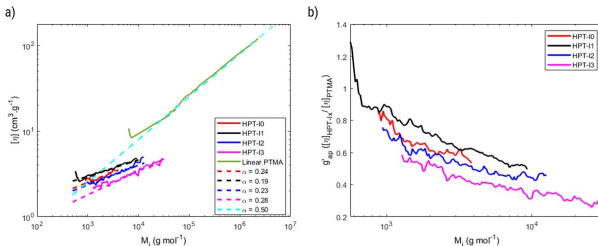
Fig. 2 (a) Double logarithmic plot of the intrinsic viscosity  $[\eta]$  against the molar mass,  $M_i$ , for the hyperbranched polymers and a linear TEMPO-based polymer analogue (PTMA) based on SEC with viscometric detection. (b) Apparent contraction factor, defined as the ratio of the intrinsic viscosity of the hyperbranched polymers to that of PTMA, as a function of molar mass.
