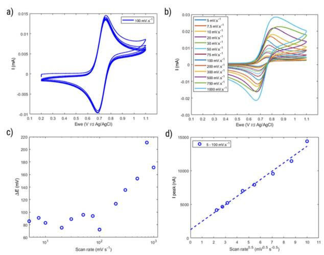
Fig. 8 (a) Cyclic voltammogram of HPT-II1Cl (5.7 mM active TEMPO) in 1.5 M NaCl aqueous solution at pH = 2.0 and at the scan rate of 100 mV s<sup>-1</sup> (six consecutive cycles). (b) First cycle voltammograms at various scan rates. (c) Peak-to-peak potential difference (obtained from the first cycle voltammograms) as a function of scan rate. (d) Oxidation peak current as a function of square root of scan rate in the reversible range (scan rates of 5 to 100 mV.  $s^{-1}$ ).
