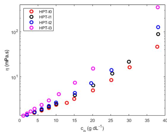
Fig. 3 Dynamic solution viscosity of the synthesized hyperbranched polymers as a function of polymer concentration in ethanol measured with a capillary ball combination.
