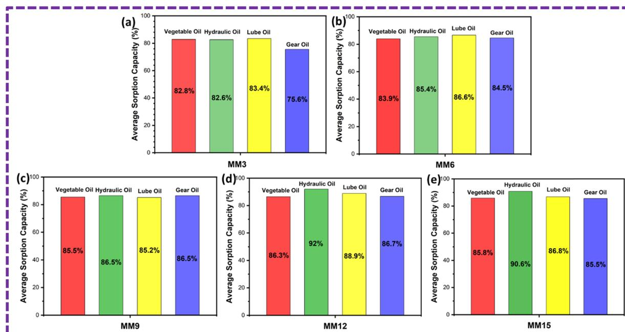
Fig. 20 Average sorption capacity after 10 cycles of the ZnS/MM/PVA-modified PU foam.
