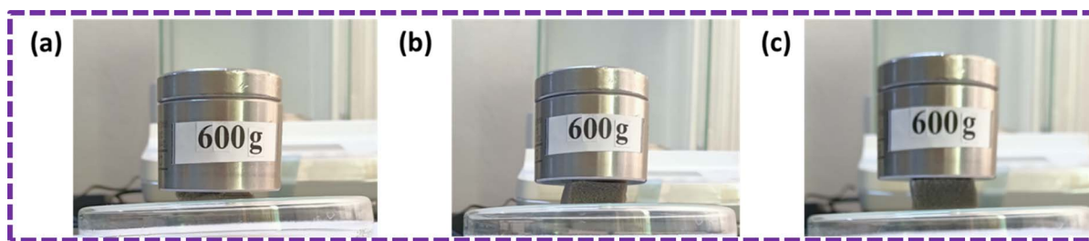
Fig. 21 Mechanical stability of the (a) pristine PU foam, (b) ZnS/CC/PVA and (c) ZnS/MM/PVA-modified PU foams.
