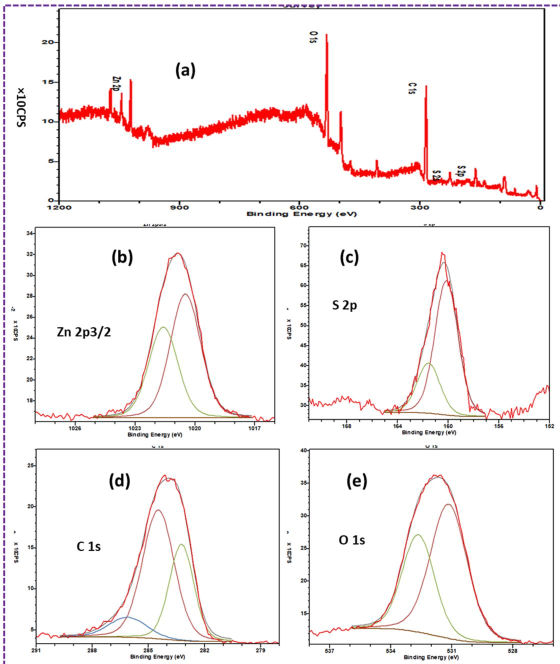
Fig. 15 XPS spectra of the dried ZnS/CC/PVA-modified PU foam: (a) survey spectrum indicating the presence of Zn, S, O, C, and (b) Zn 2p<sub>3/2</sub>, (c) S 2p, (d) O 1s, and (e) C 1s, respectively.
