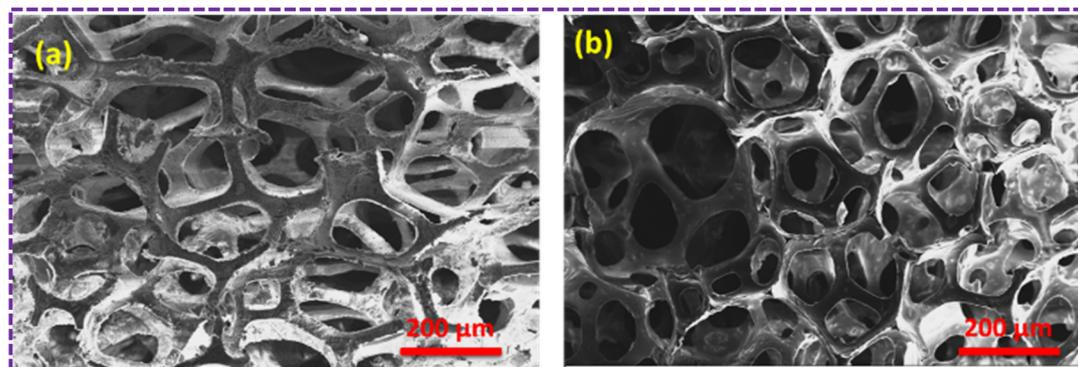
Fig. 5 (a) SEM image of the ZnS/CC/PVA-modified PU foam before the oil sorption test. (b) SEM image of the ZnS/CC/PVA-modified PU foam after oil sorption.
