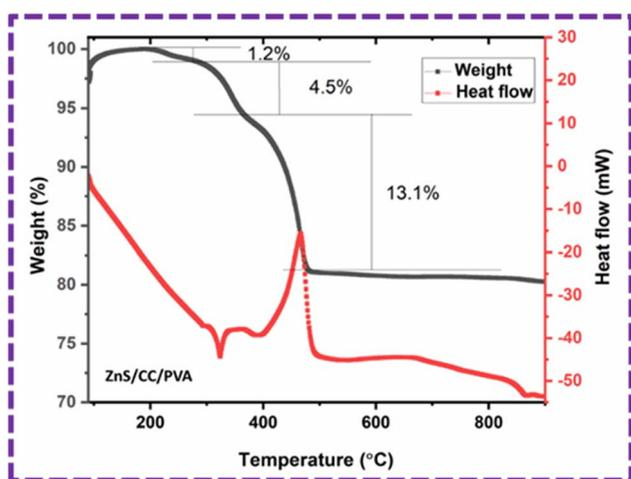
Fig. 13 TGA (weight%) and DSC (heat flow) graph of the ZnS/CC/PVA composite in the temperature range of 49–900 °C.
