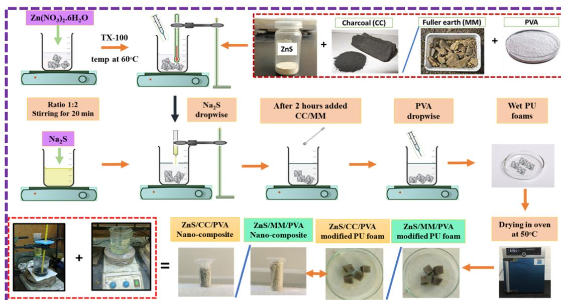
Fig. 1 Schematic representation of the ZnS/CC/PVA and ZnS/MM/PVA nanocomposites-modified PU foams.
