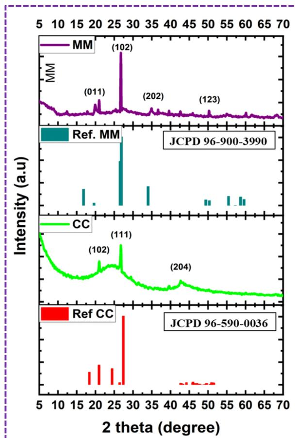
Fig. 3 XRD patterns of CC and MM.
