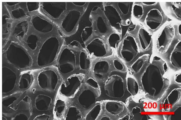
Fig. 4 FE-SEM image of the pristine PU foam.
