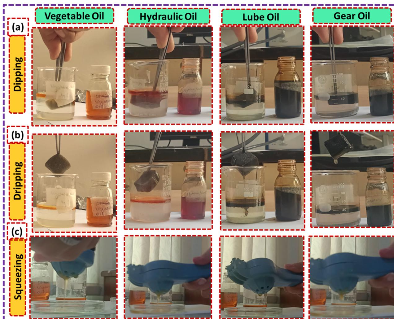
Fig. 16 Oil sorption capacity test (g g<sup>-1</sup>) of the modified PU foam: (a) dipping, (b) dripping, and (c) squeezing.
