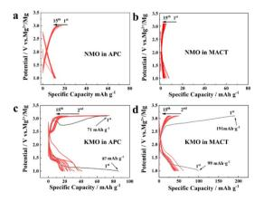
Fig. 3 Electrochemical performances of NMO and KMO in magnesium batteries. The galvanostatic charge/discharge curves of NMO in (a) APC and (b) MACT electrolytes. The galvanostatic charge/discharge curves of KMO in (c) APC and (d) MACT electrolytes.
